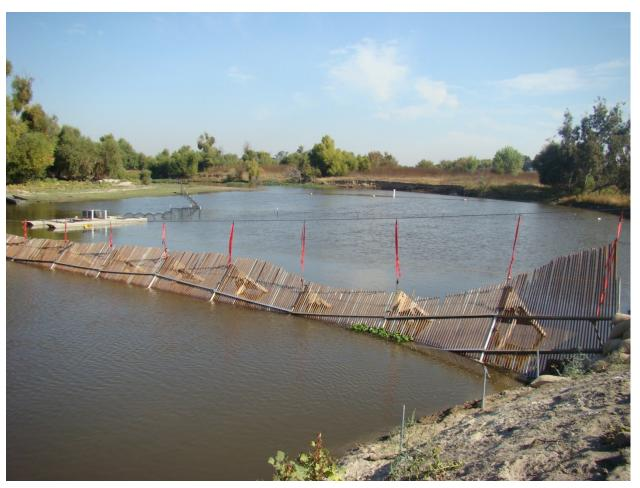
Figure 6: fyke trap with floating trap downstream of Hills Ferry Barrier
