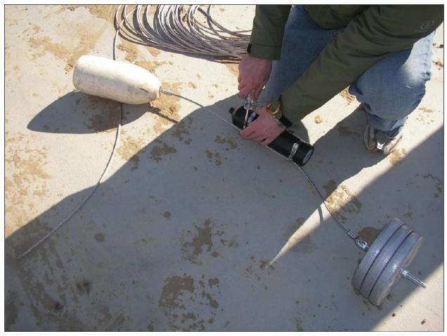
Figure 8: Vemco receiver with flat weights and buoy
