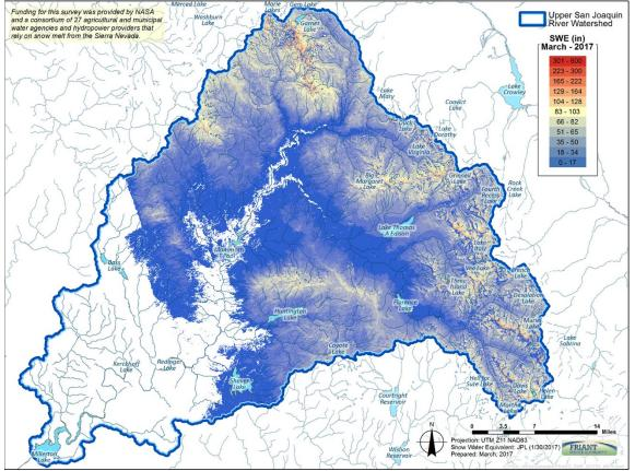
ASO produces snow water equivalent measures through a combination of LIDAR and ground-based snow density measures. The resolution is extremely fine detailed, capturing features and trends across the landscape that cannot be discerned from a handful of station or snow course measures.
