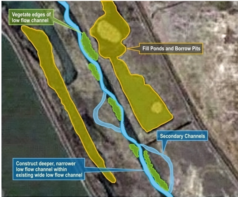
Figure 5-6. Alternative 2 – Example of Channel Excavation in the Eastside Bypass
