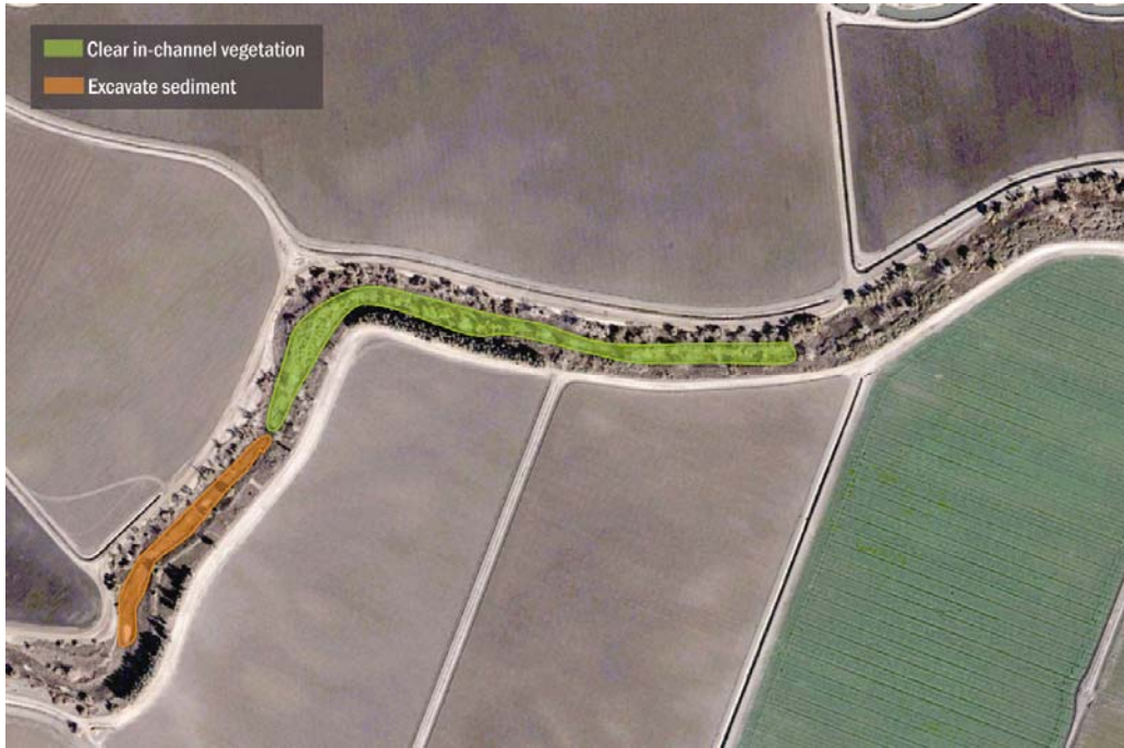
Figure 5-5. Alternative 2 – Example of Channel Excavation and Vegetation Clearing in the San Joaquin River
