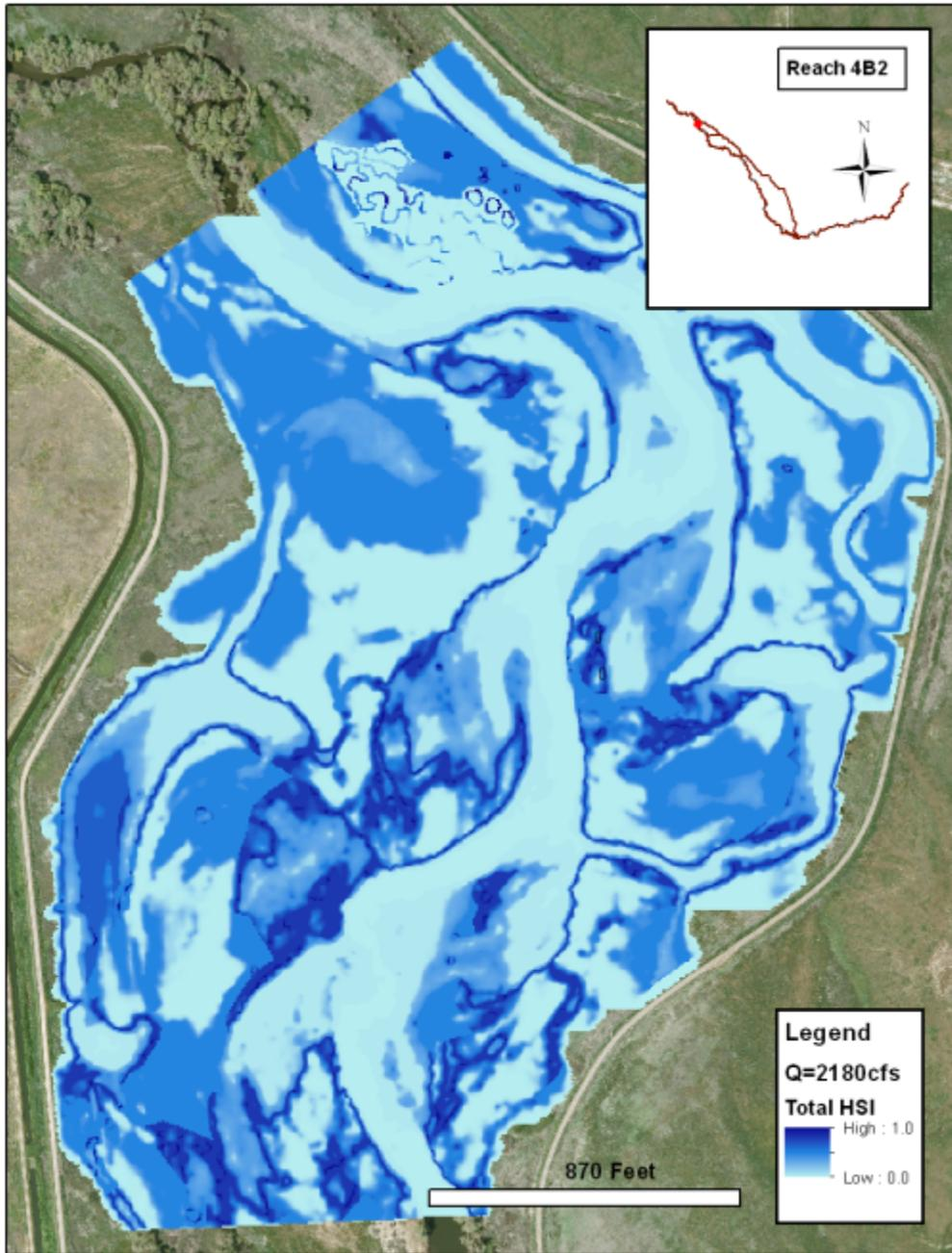
Figure 28. Distribution of calculated total HSI in Reach 4B2 for simulation "normal" water year type.
