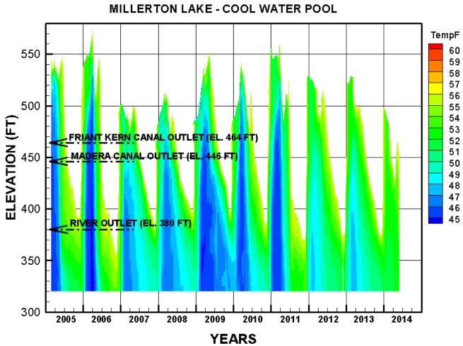
Note: For this plot, cool water is defined to be water temperatures below 56 °F. This plot illustrates a clear trend that the cool water pool volume and temperature is greatly reduced in 2012, 2013, and 2014. With current drought conditions, May 2014 cool water pool temperatures are about 3.8°F warmer than in May 2013.
