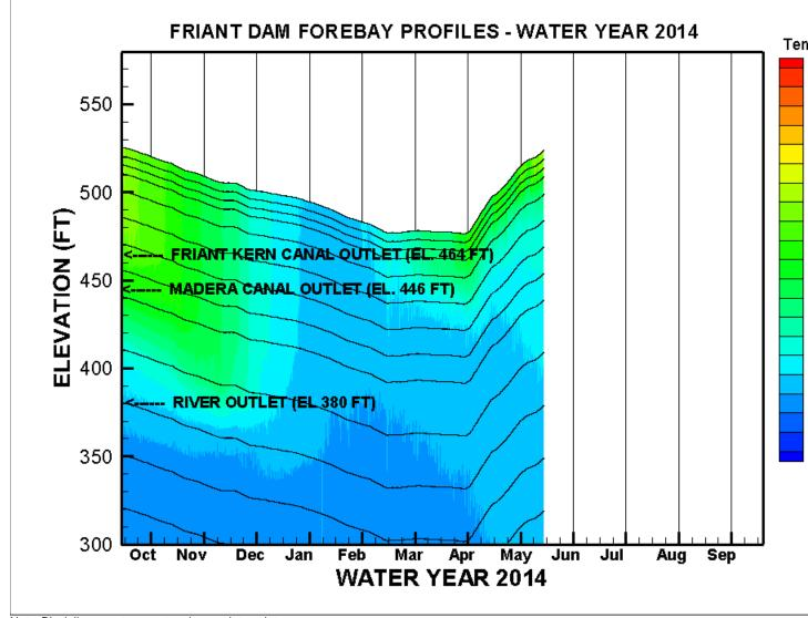
Note: Black lines are temperature logger data points. **Figure 2. Friant Dam Forebay Water Temperature Profile Data for Water Year 2014**
