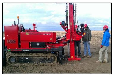
Figure 1: Drill rig creating a bore hole for shallow well testing.
