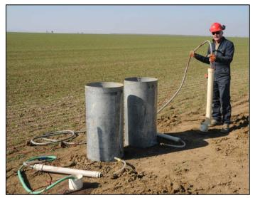
Figure 2: Shallow well pump-in test (left), and ring permeameter test (right)
