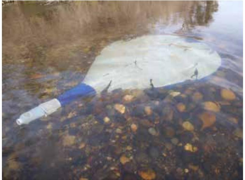
Figure 2: Emergence trap placed over redd in Reach 1 of the San Joaquin River during 2013.
