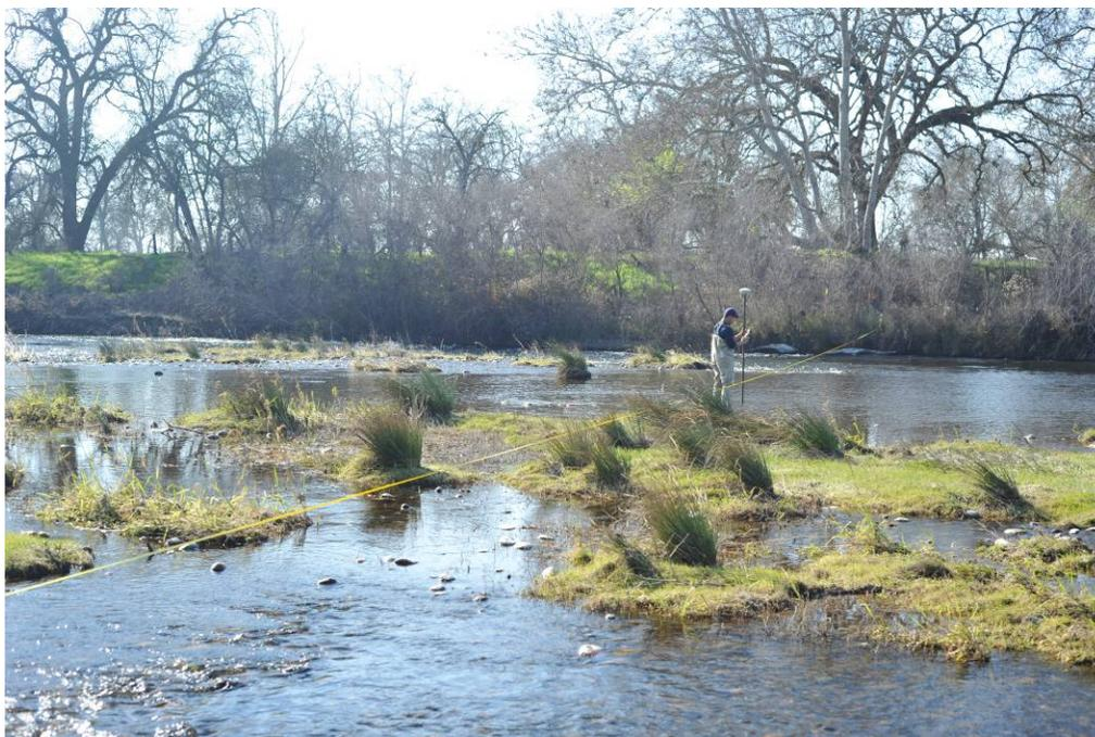
Note: The yellow tape is stretched between monument stakes on both banks and the rover rod is held plumb while placed tangential to the tape at each survey point.
