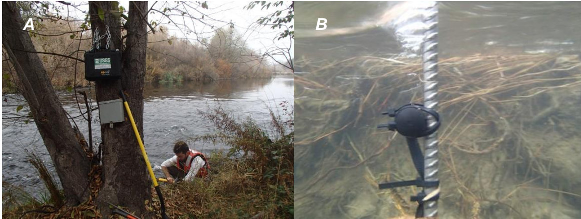
Figure 1. Hydrophone Installation on the San Joaquin River (A), Close-up View of Submerged Hydrophone Mounted Near Bank (B)
