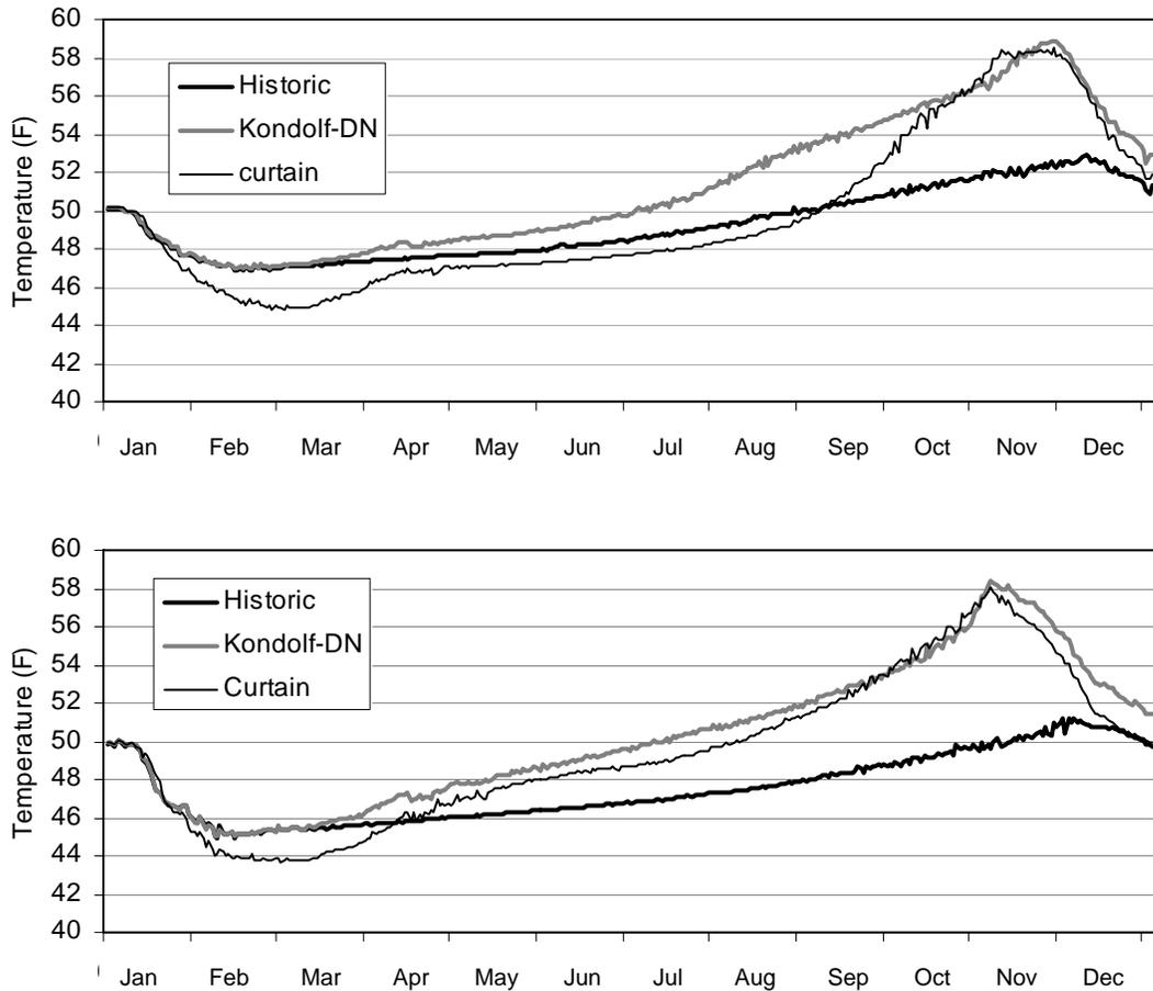
**Figure 6. Simulated Millerton Reservoir Friant Dam river outlet release temperatures for historic, Kondolf proposed Dry-Normal hydrograph, and Kondolf proposed Dry-Normal hydrograph with upstream temperature control curtain: 2003 (top) and 2004 (bottom)**
