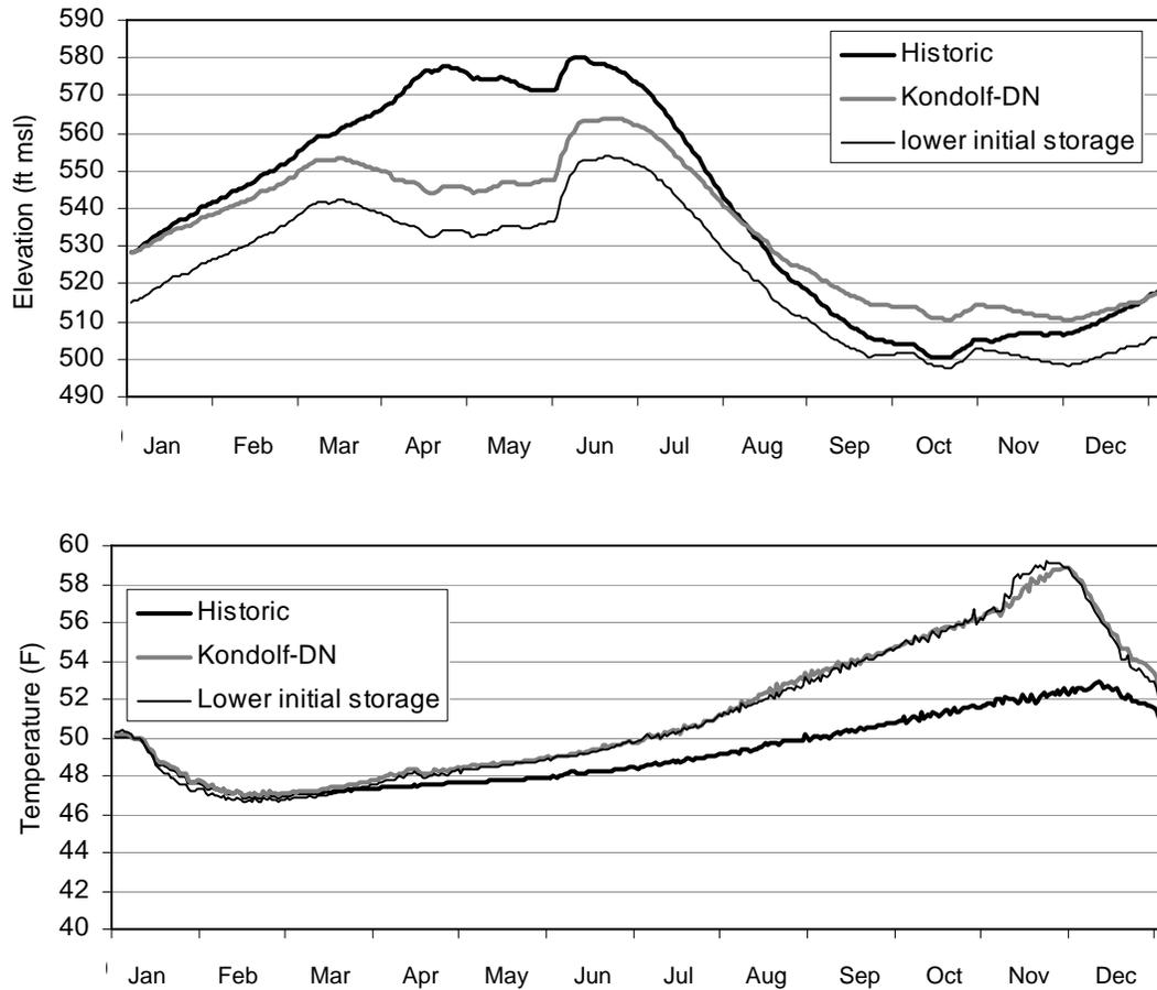
**Figure 4. Simulated Millerton Reservoir water surface elevation (top) and Friant Dam river outlet release temperatures (bottom) for historic, Kondolf proposed Dry-Normal hydrograph, and Kondolf proposed Dry-Normal hydrograph with lower initial reservoir storage: 2003**
