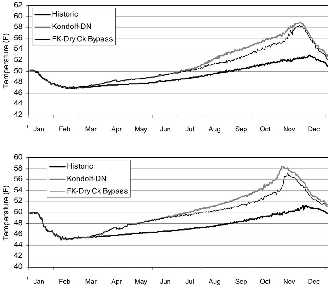
**Figure 7. Simulated Millerton Reservoir Friant Dam river outlet release temperatures for historic, Kondolf proposed Dry-Normal hydrograph, and Kondolf proposed Dry-Normal hydrograph with release via Friant Kern Canal and Dry Creek: 2003 (top) and 2004 (bottom)**
