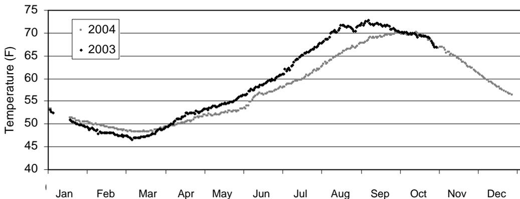
**Figure 8. Friant-Kern Canal simulated outlet temperatures, 2003 and 2004 (where series of data points are absent, no canal flow on those days)**
