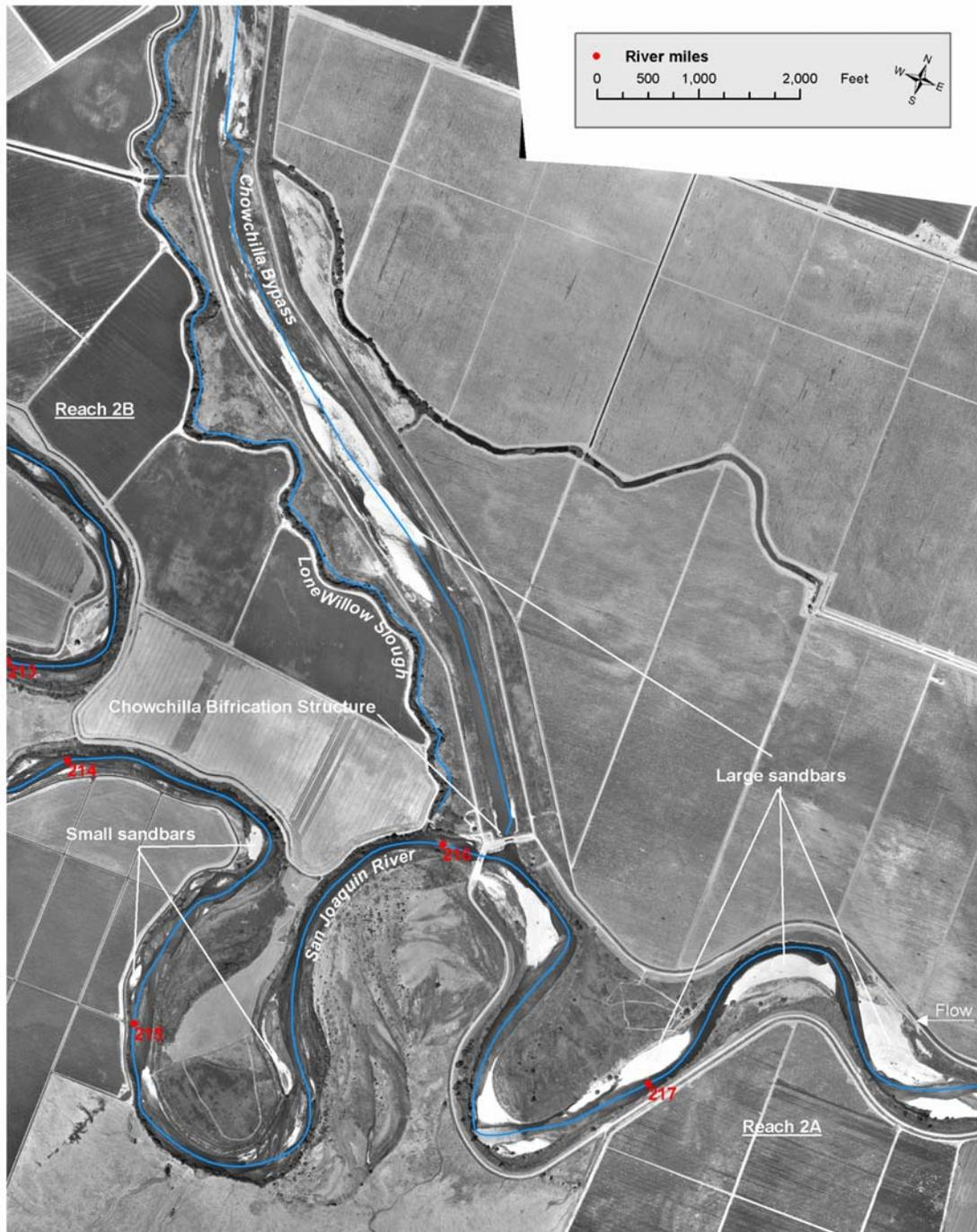
**Figure 3.1-9. Restoring sediment supply and routing in Reach 2B.** Current operation of the Chowchilla Bifurcation Structure directs a higher proportion of flow, and therefore sediment, into the Chowchilla Bypass during high flow events. As a result, the sediment supply to Reach 2B is reduced.
