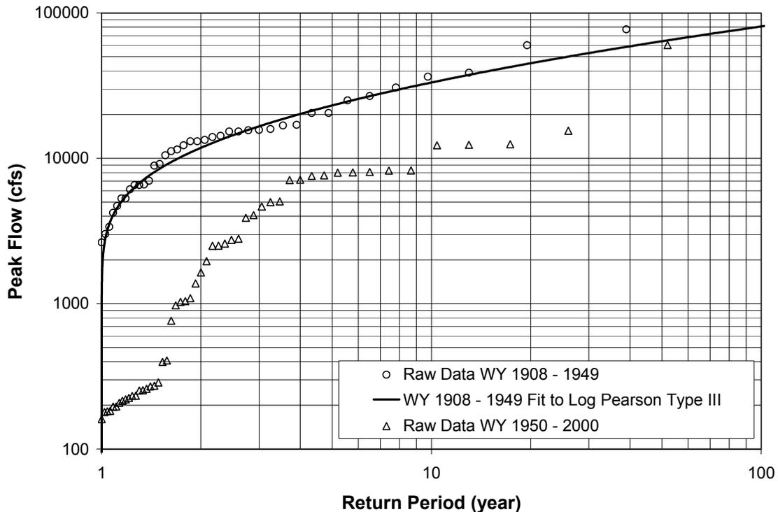
**Figure 3.1-3. Peak flow recurrence in Reach 1 of the San Joaquin River.** A pre-dam flow of 20,000 cfs corresponds with a return period of 4 years, and a discharge of 40,000 cfs represents a 15-year return period. This analysis represents flow conditions at the USGS Gauge at Friant Dam (no. 11251000).
