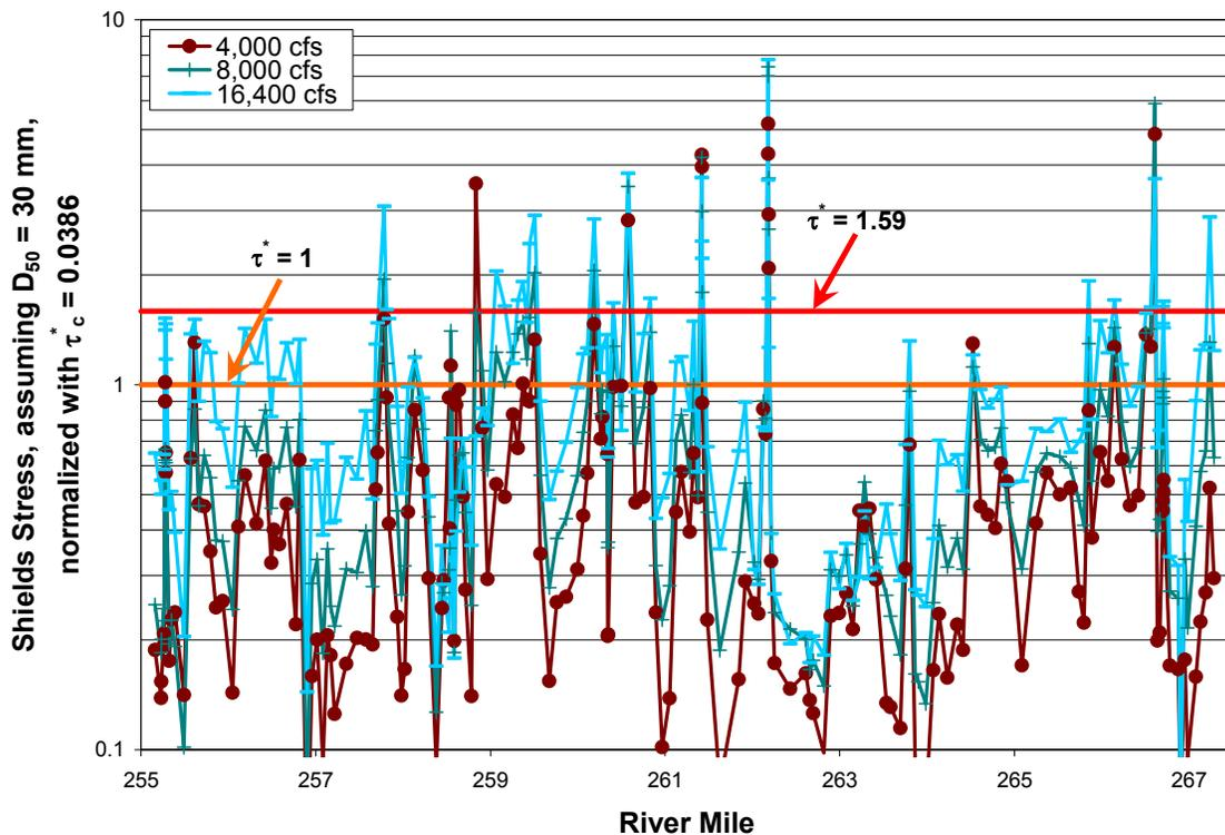
**Figure 3.1-6. Sediment mobility and scour for a median grain size of 30 mm using local shear stresses.** These results are based on MEI HEC-2 results, a median grain size of 30 mm, and a critical Shields stress of 0.0386. Introducing finer sediment to Reach 1A will not effectively restore general bedload routing, because flows higher than the managed release capacity of Friant Dam will still be required to scour coarse sediment from Reach 1 pools.
