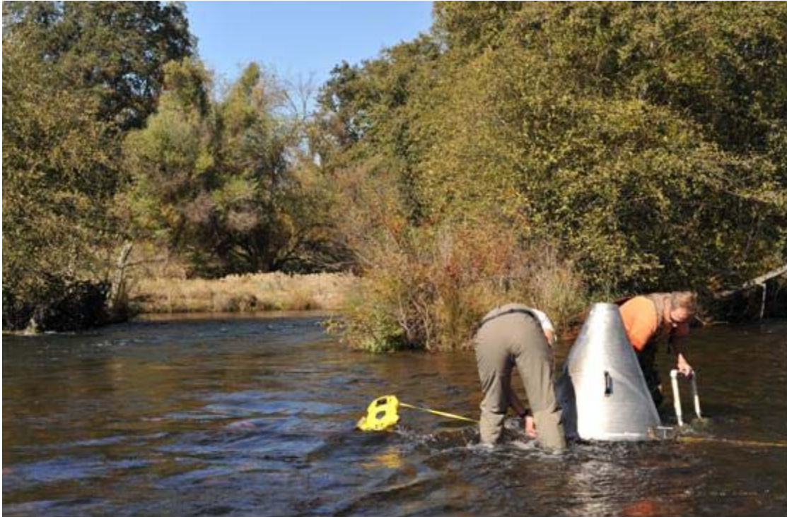
Figure 13 - Photoscope in use during photo-survey of cross-section 3; viewed looking upstream.
