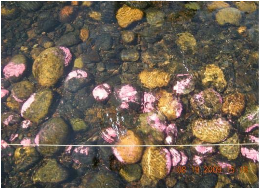
Figure 11 – An example of the bed’s condition before and after tracer painting (XS-3, approx bin 30-31)
