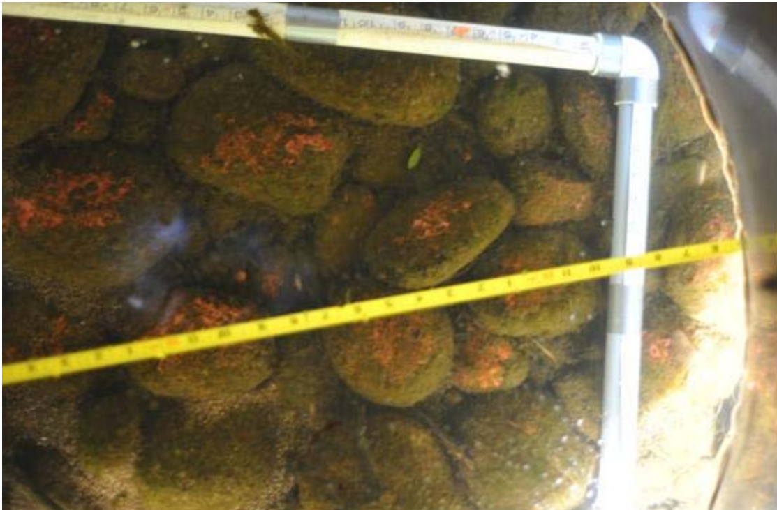
Figure 14 - An example of a photo of the bed shot through the photoscope. The yellow tape indicates the position along the cross-section. The white frame serves as a scale to measure gravel diameters.
