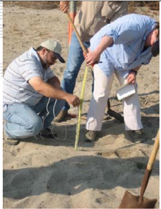
Photo 4. Measuring excess chain above ground
