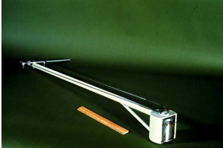
1 2 3 Figure D-1. US RBMH-80 – Hand Held Rotary Scoop Bed Material Sampler
