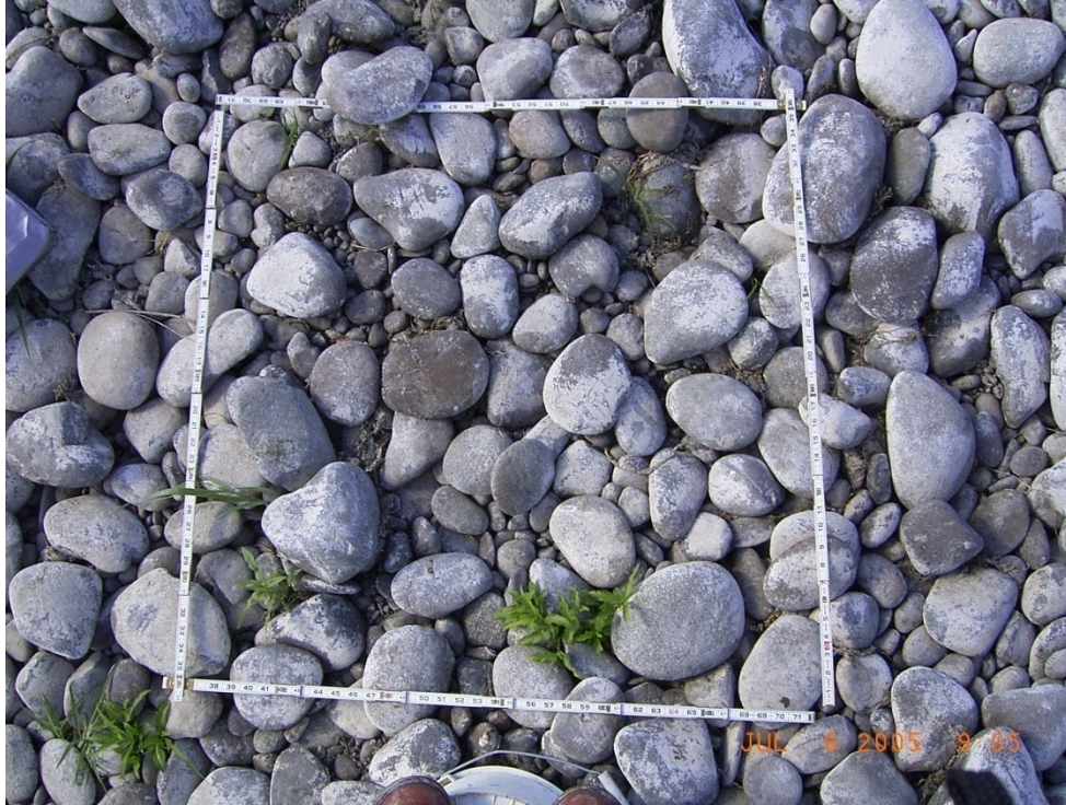
Figure D-2. Rectangular Area Defined for Photogrammetric Sampling Above Water
