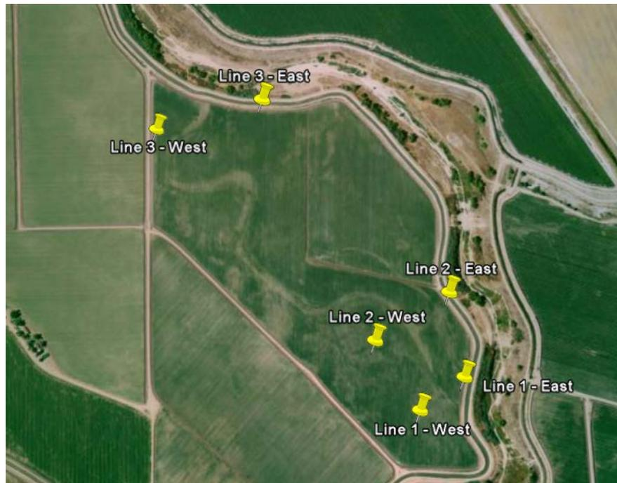
**Figure 1: Property 1 Electrical Resistivity Tomography Lines**
