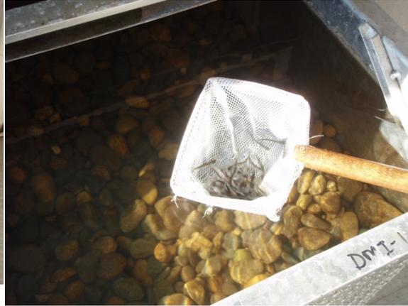
**Figure 2. Inside view of Deep Matrix Incubator gravel and emerging fry.**
