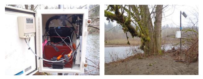
Figure 1a,b. Hydrophone installation on the Cedar River, Washington. a.) interior of the installation enclosure showing the digital timer, computer, geophone battery and charger; b.) location of the hydrophone installation (the pipe containing the cable to the hydrophone receiver is underground). Photo by M. Marineau (2/2011).
