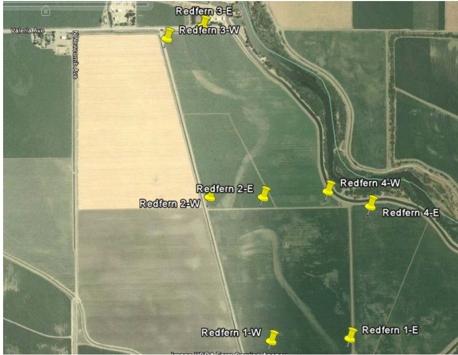
Figure 2: Property 2 Electrical Resistivity Tomography Lines
