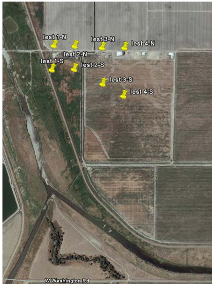
Figure 3: Property 3 Electrical Resistivity Tomography Lines
