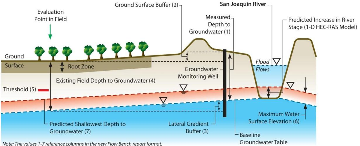
**Figure 2: Conceptual Model for Increase in Stage Method**
