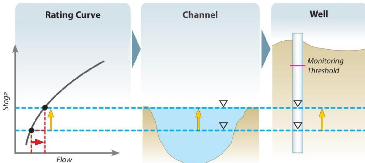
**Figure 1: Conceptual Model of 1:1 Relationship between River Stage and Groundwater Level**
