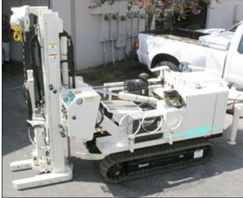
1 2 Figure 3-1. 3 Tractor Mounted Hydraulic Probe (Geoprobe 6610 DT)
