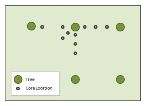
Figure 3-2. Example Layout of Core Locations within a Study Site
