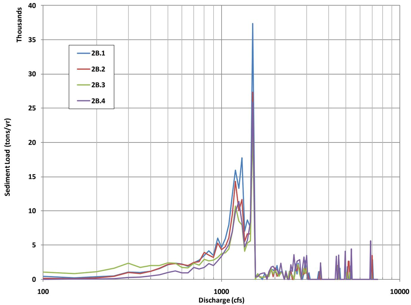
Figure 14. Average annual quantity of sediment transported by increments of flow between 100 and 8,000 cfs, based on the baseline-conditions mean day flow-duration curve and the bed-material transport capacity rating curves for each subreach.
