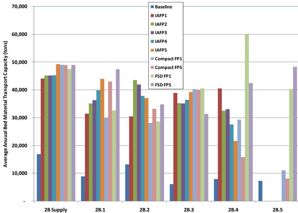
Figure 8. Average annual bed-material transport capacity in Subreaches 2B.1 through 2B.5 under baseline and project alternatives.
