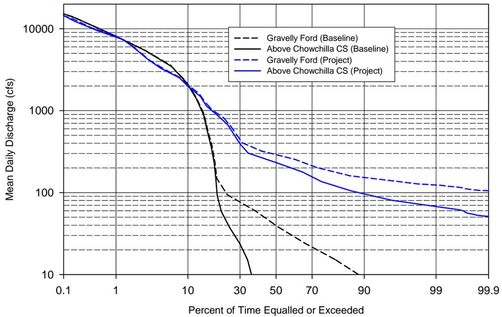
Figure 7. Mean daily flow-duration curves in the San Joaquin River at Gravelly Ford and above the Chowchilla Bypass Control Structure under baseline and project conditions, based on the 23-year record of estimated mean daily flows.
