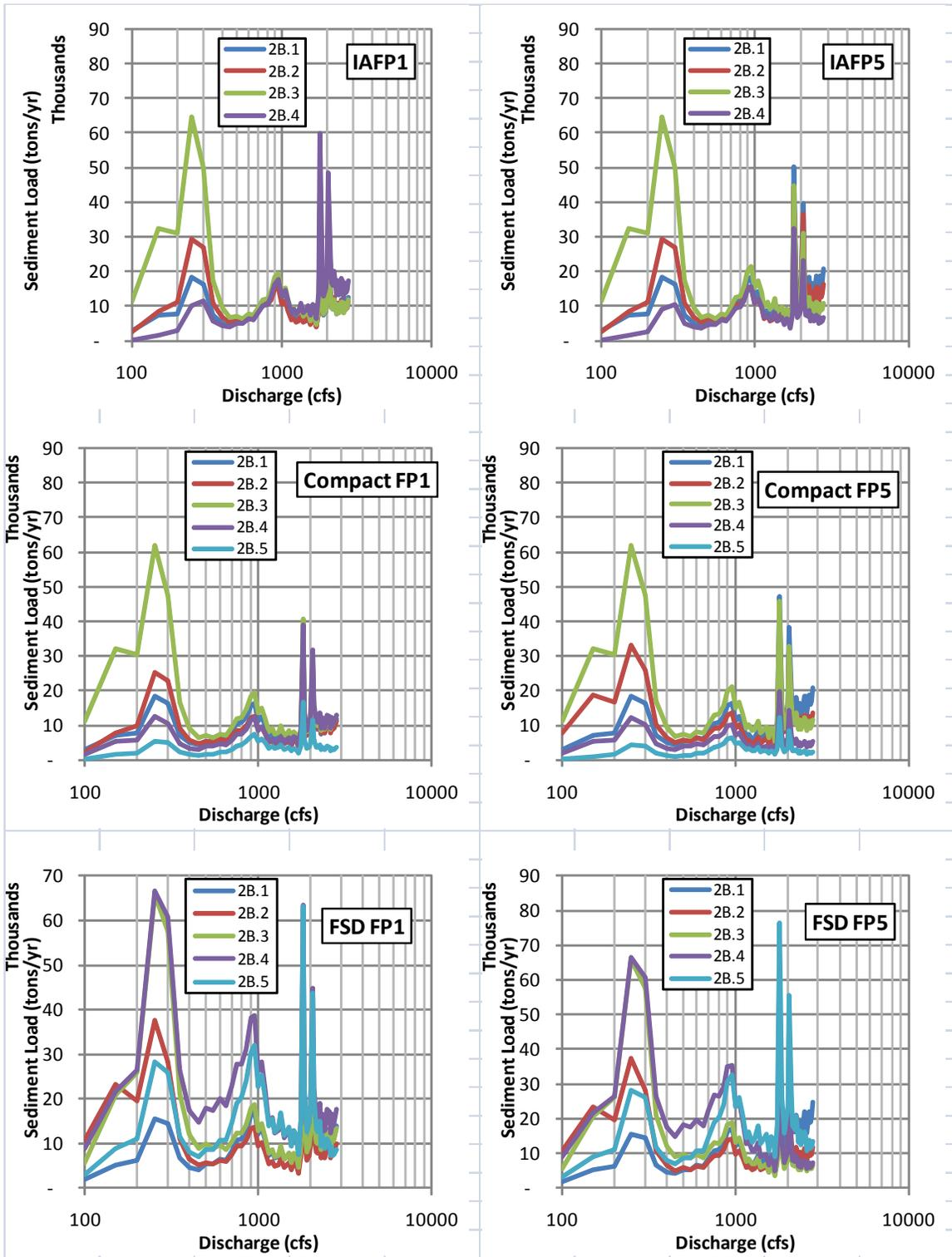
Figure 15. Average annual quantity of sediment transported by increments of flow between 100 and 8,000 cfs for the various Mendota Pool Bypass Options and the narrow (FP1) and wide (FP5) setback options, based on the project-conditions mean day flow-duration curve and the bed-material transport capacity rating curves for each subreach.
