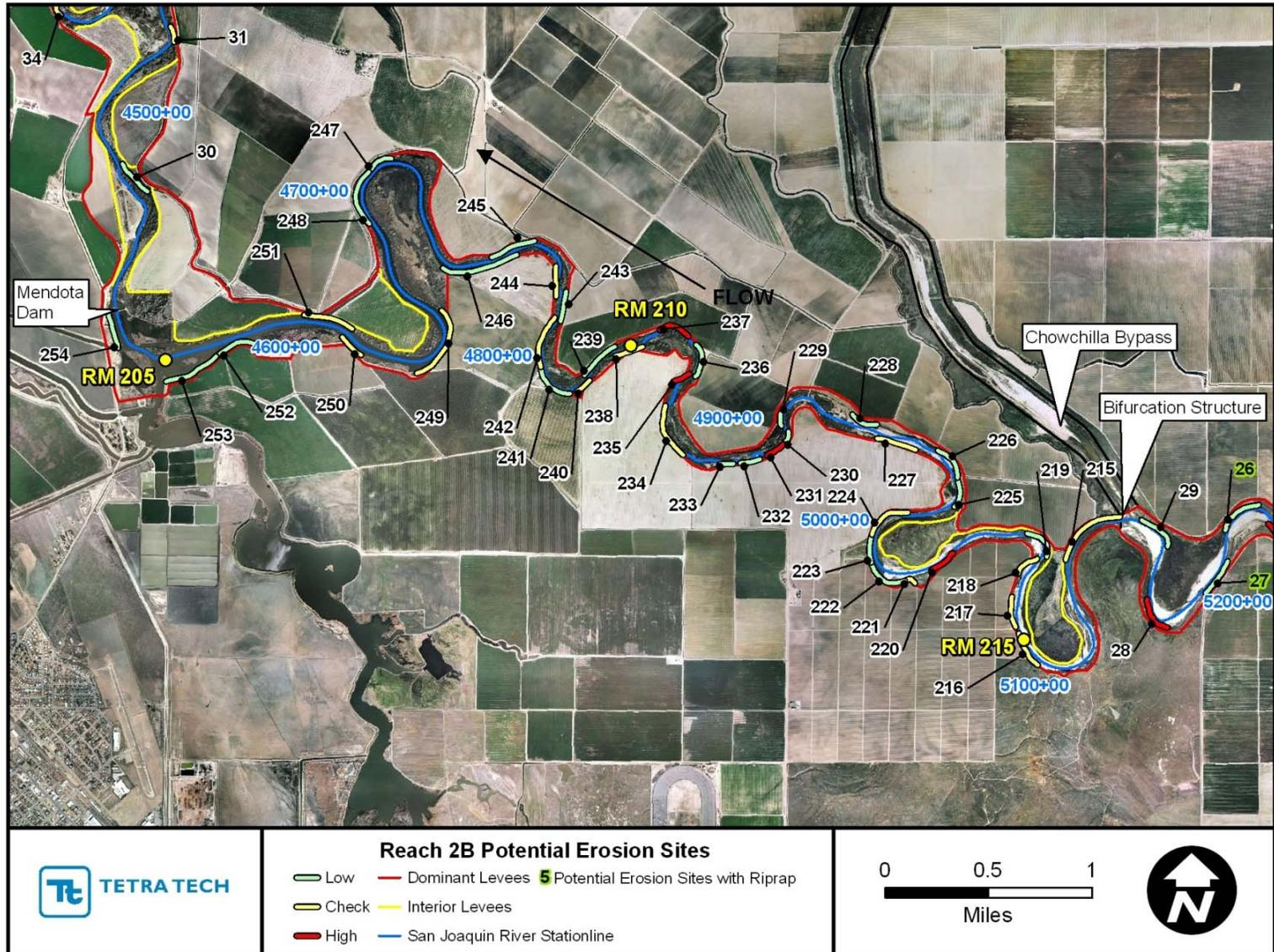
Figure 10. Aerial map showing potential lateral bank erosion sites in Reach 2B.
