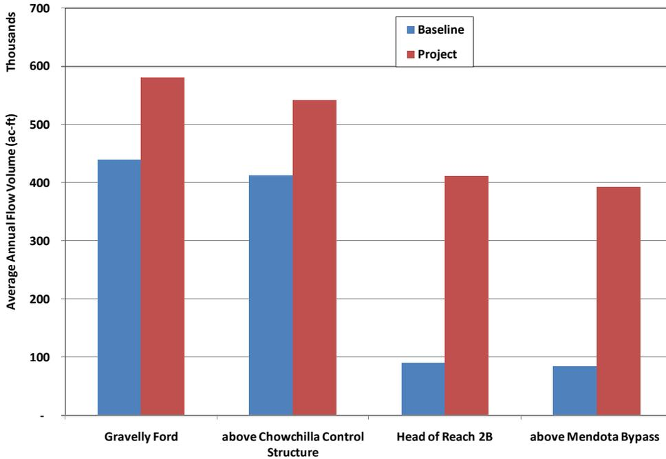
Figure 5. Average annual flow volume at various locations in Reaches 2A and 2B under baseline and project conditions based on the daily disaggregated flow records used for the analysis.
