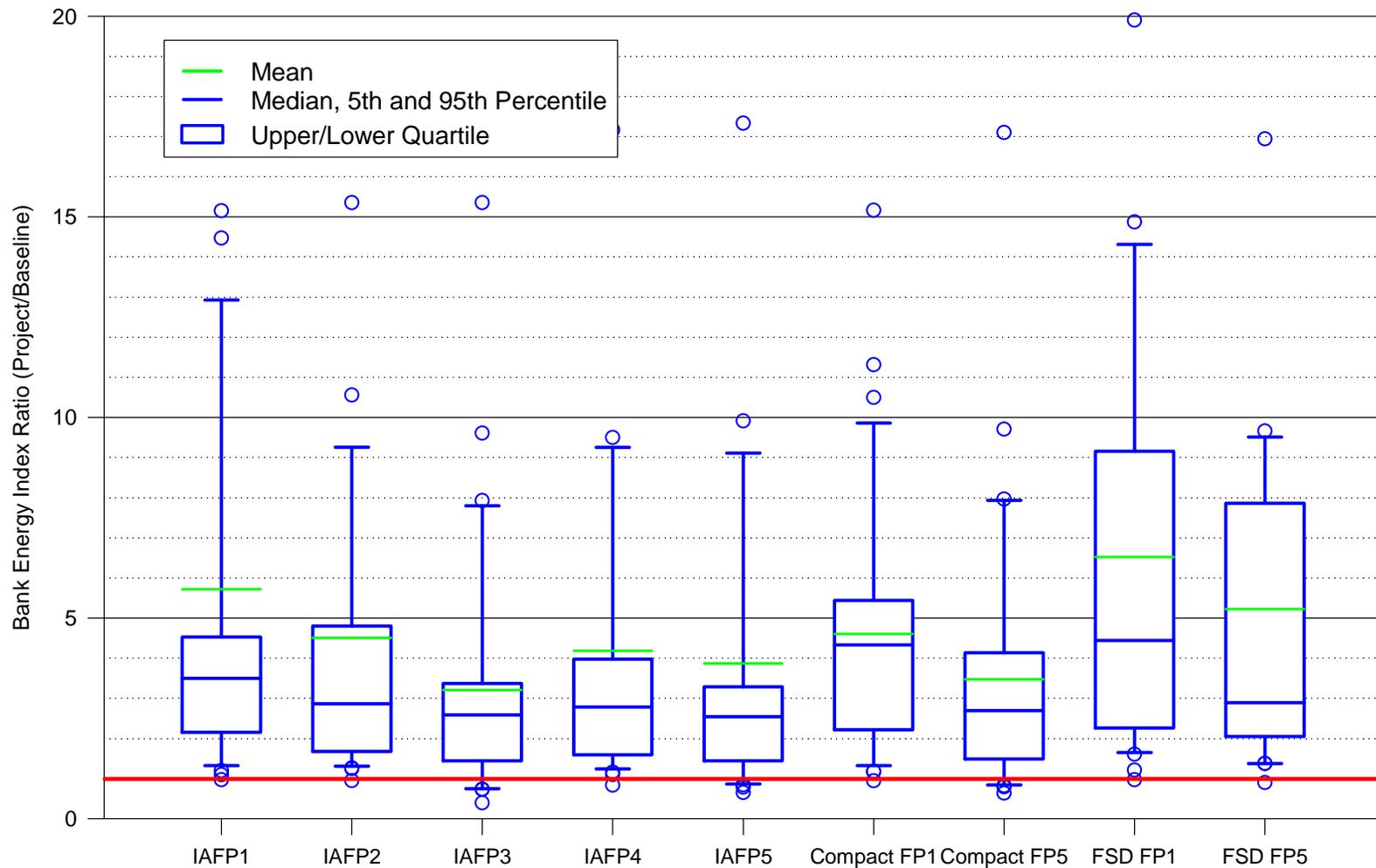
Figure 12. Statistical summary of ratio of Bank Energy Index (BEI) under project conditions to the BEI under baseline conditions for the 33 potential erosion sites in Reach 2B upstream from the proposed Mendota Bypass Channel Control Structure.
