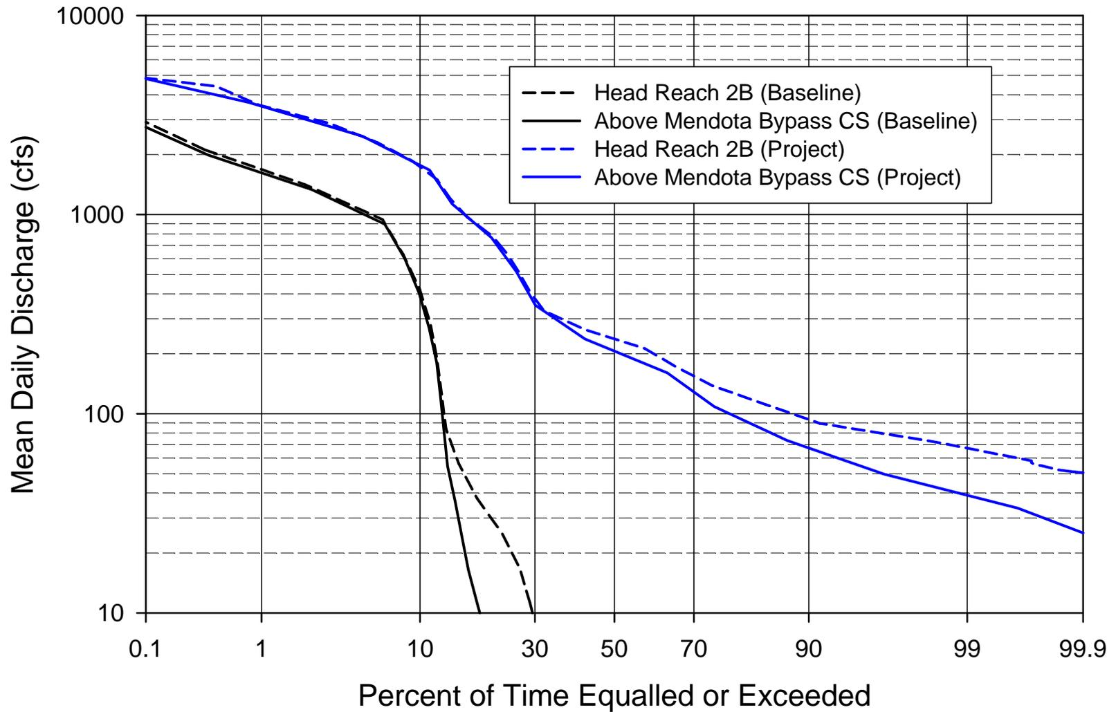
Figure 11. Mean daily flow-duration curves in the San Joaquin River at the head of Reach 2B and above the proposed Mendota Bypass Control Structure under baseline and project conditions, based on the 23-year record of estimated mean daily flows.
