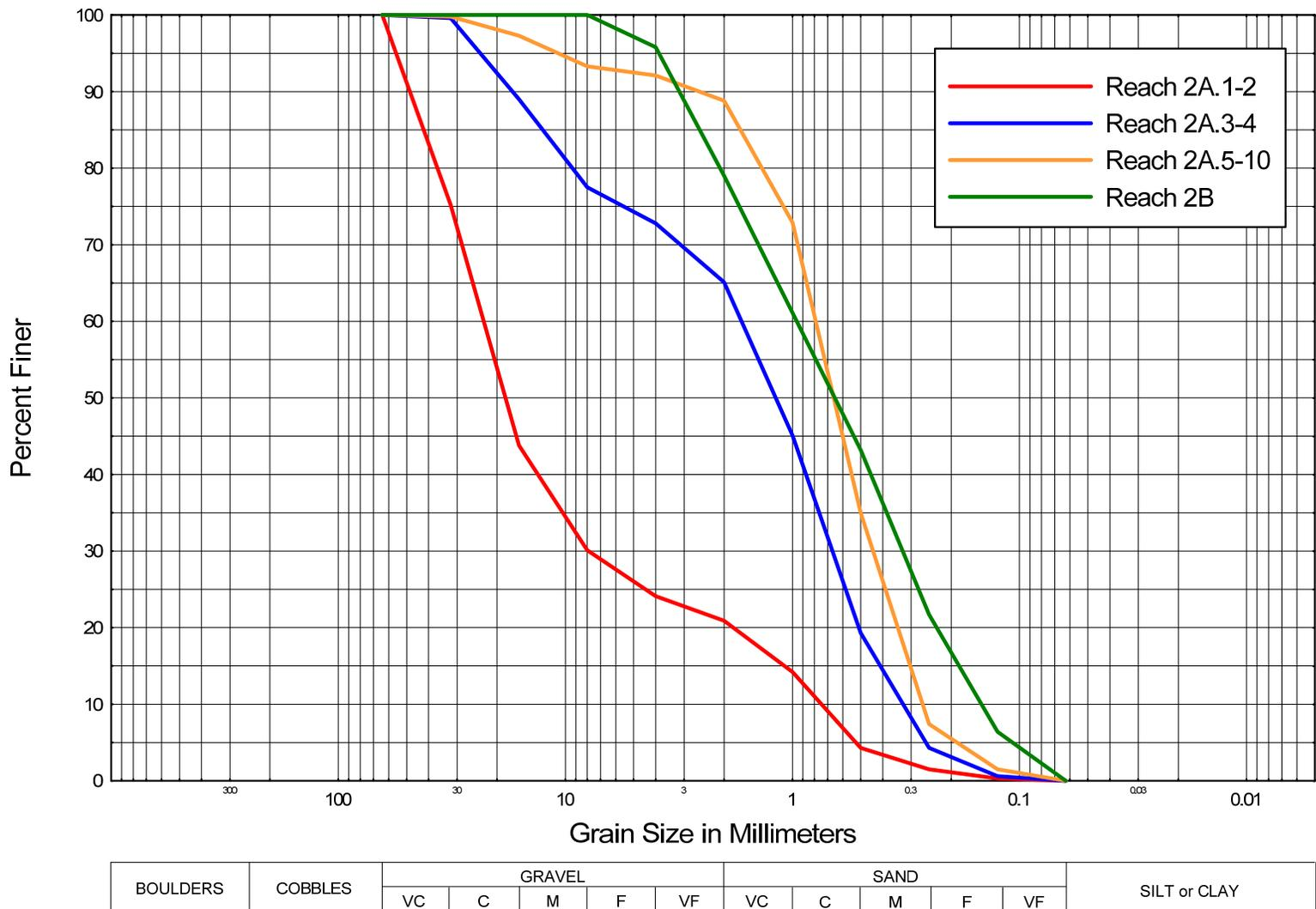
Figure 4. Representative bed-material gradations for the lower end of Reaches 2A and 2B used in the sediment-transport analysis.
