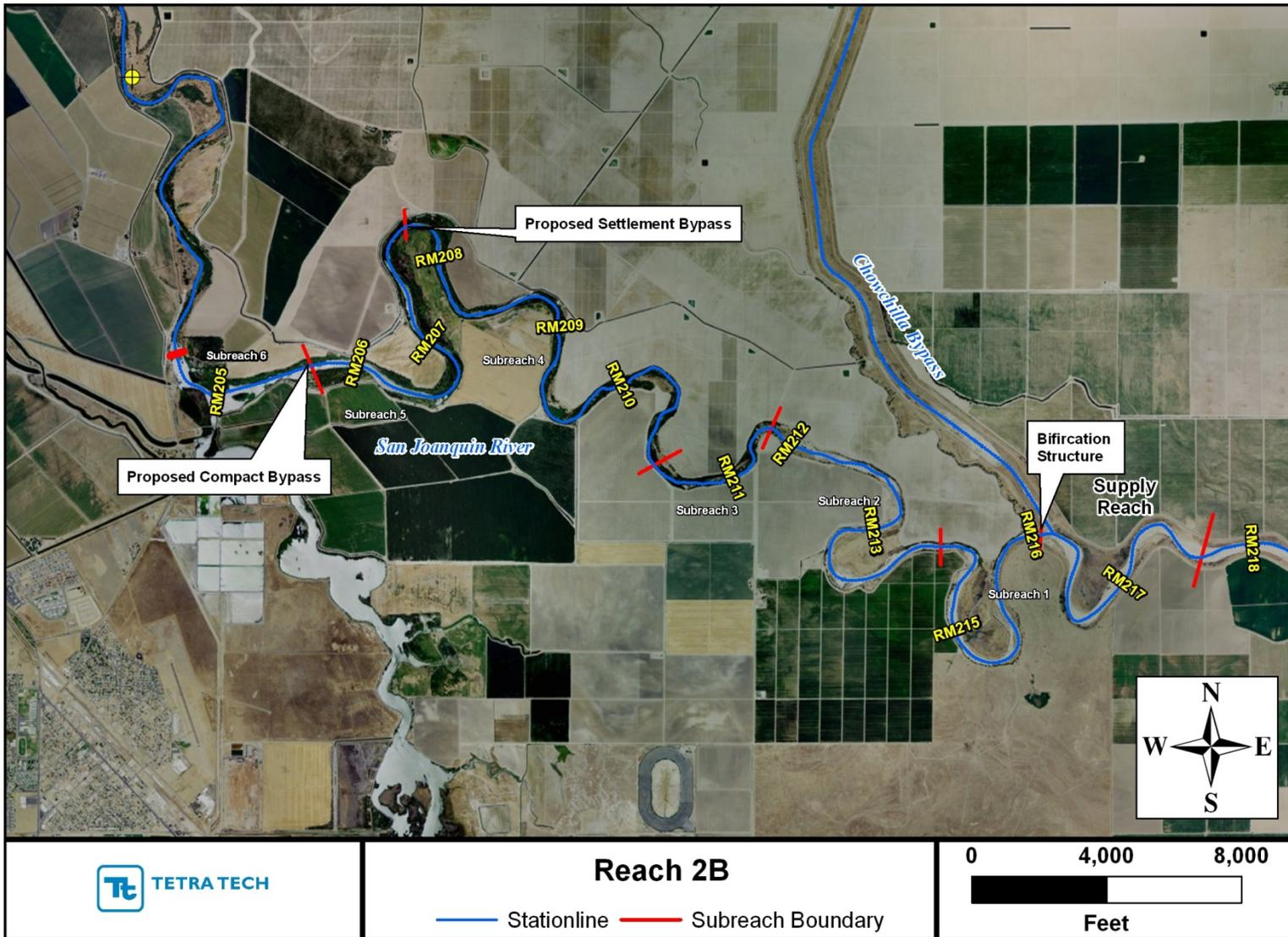
Figure 1. Planview of San Joaquin River Reach 2B showing the subreach delineations used for the vertical stability analysis.
