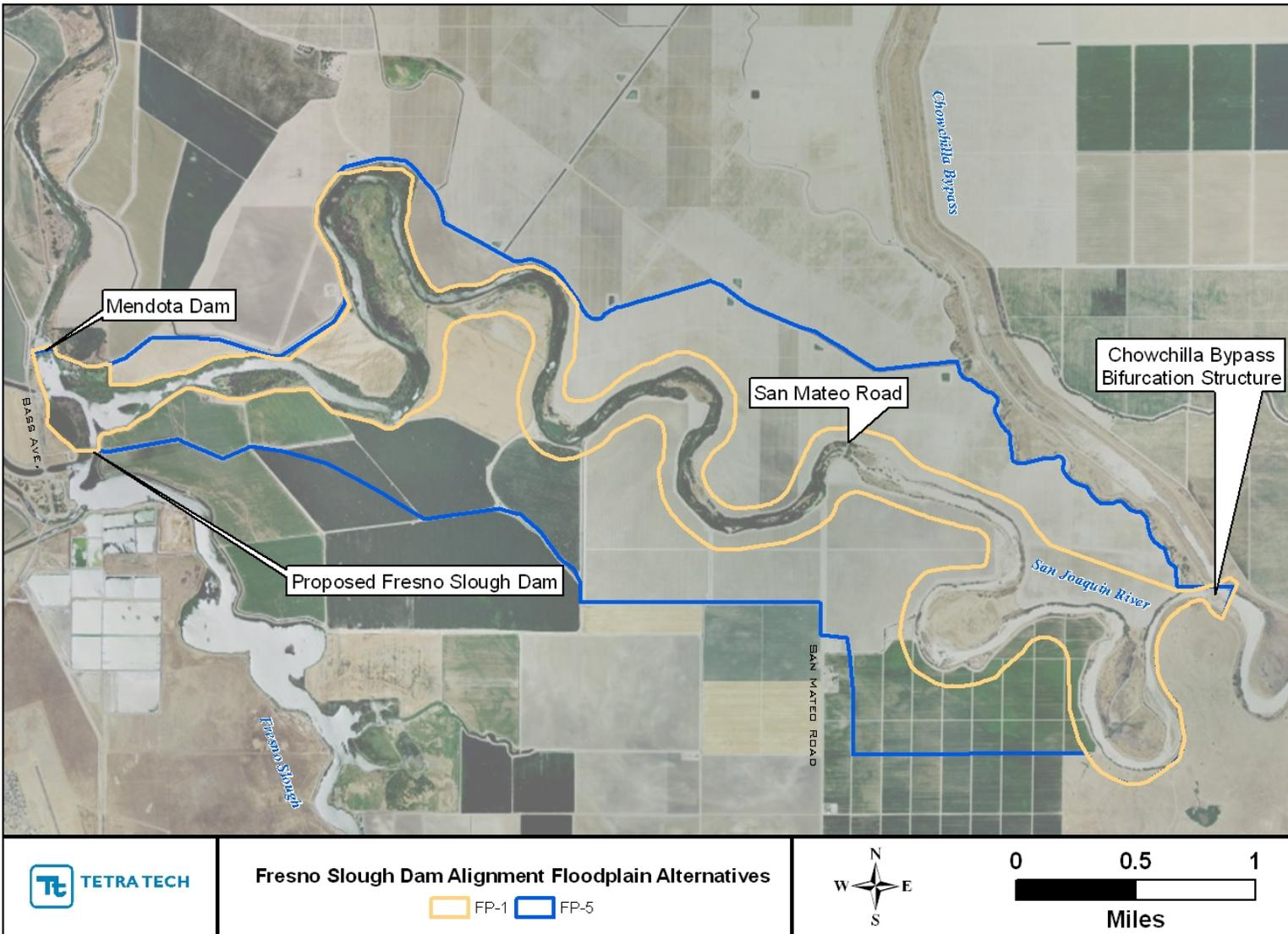
Figure 2c. Planview of Reach 2B showing the various levee setback alternatives associated with the Fresno Slough Dam Alternative.
