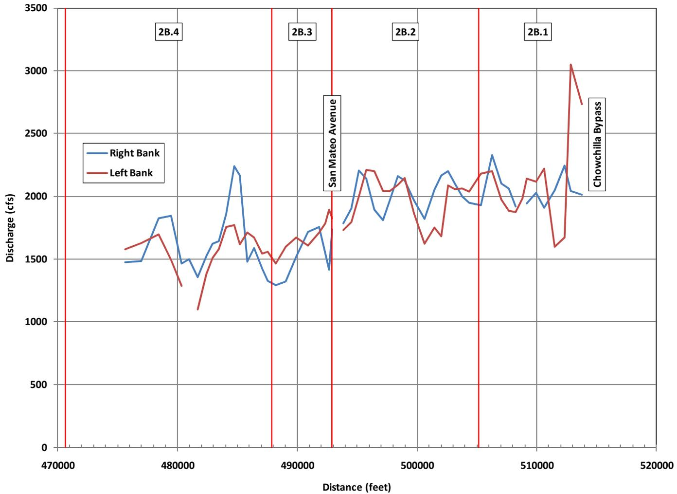
Figure 16. Bankfull discharge in the portions of Reach 2B near the head, and upstream from, the normal backwater effect of Mendota Dam, based on the ground elevations outside the interior levees.
