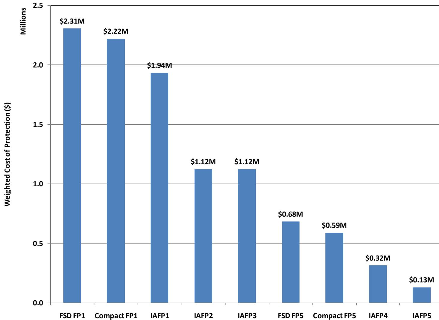
Figure 13. Estimated risk-weighted cost of providing lateral erosion protection for the range of Mendota Bypass and levee setback alternatives for Reach 2B.
