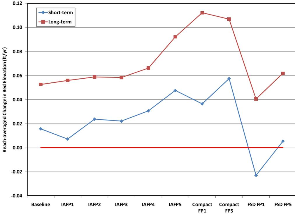
Figure 9. Average annual change in bed elevation in Reach 2B under baseline and a range of project conditions.
