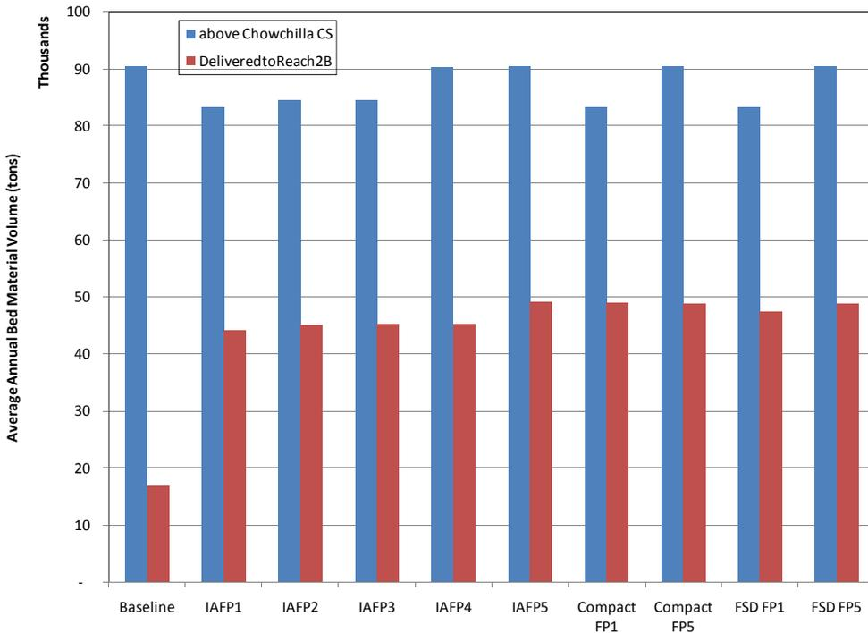
Figure 6. Average annual bed material transport capacity in the approximately 1.7-mile portion of Reach 2A just upstream from the Chowchilla Bypass Control Structure under baseline and various levee-setback and Mendota Dam Bypass Alternatives. Also shown is the estimated, average annual bed material load delivered through the Control Structure into Reach 2B.
