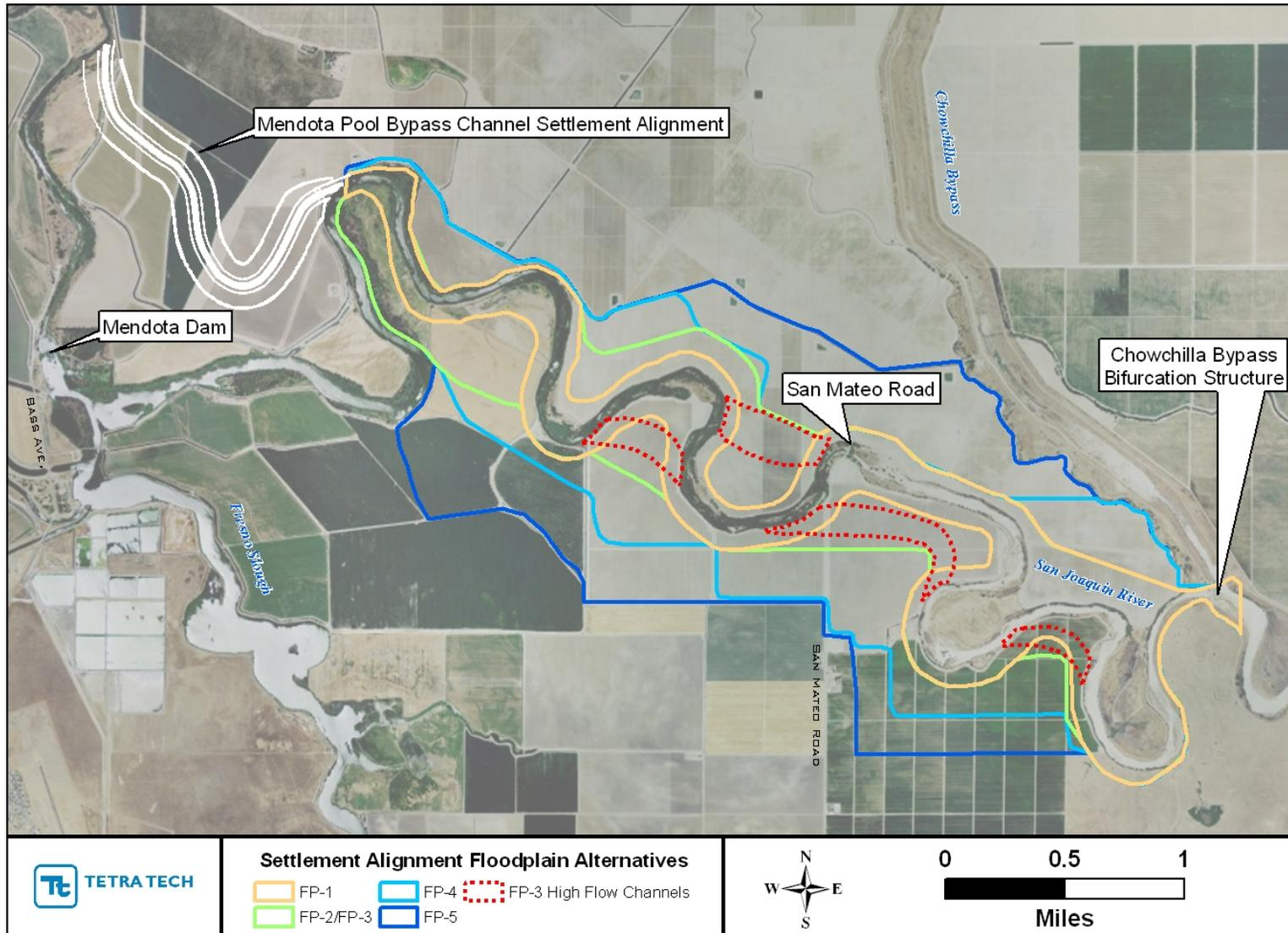
Figure 2a. Planview of Reach 2B showing the various levee setback alternatives associated with the Mendota Pool Bypass Channel Settlement Alignment.
