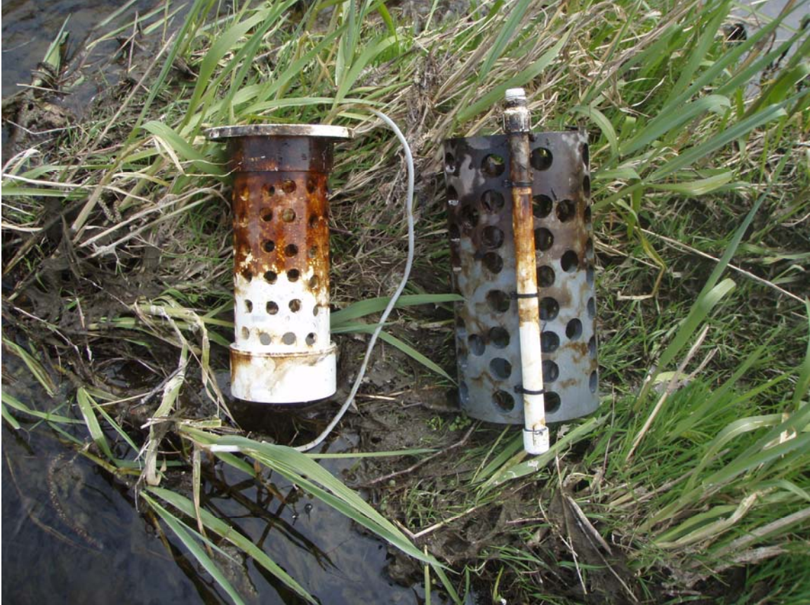
Figure 2. Photo showing hyporheic sampler (left) and sleeve (right) with attached piezometer.
