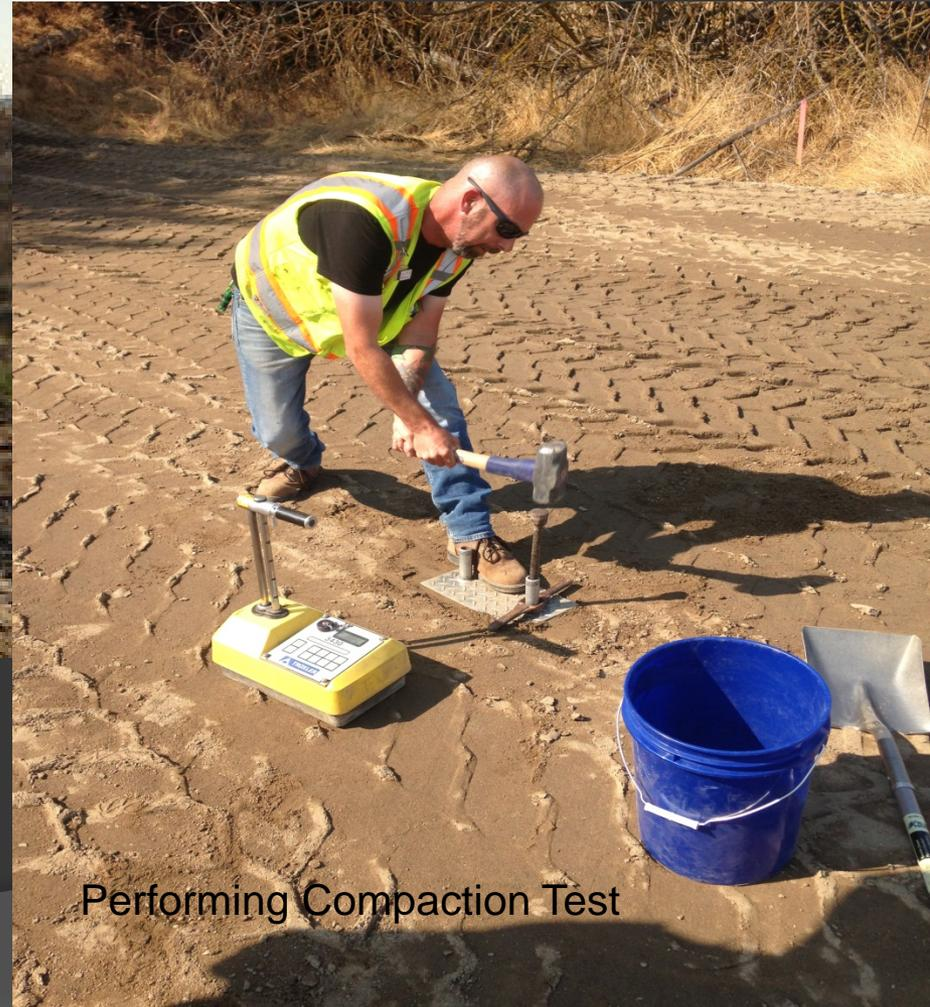
Performing Compaction Test
