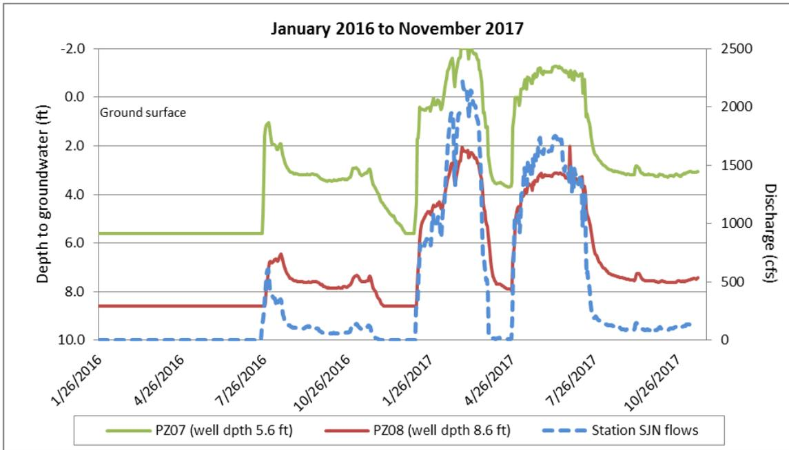
**Figure 15.** Depth to groundwater at wells PZ-7 and -8 and San Joaquin River discharge at gauge SJN from January 2016 to November 2017 in Reach 2B.
