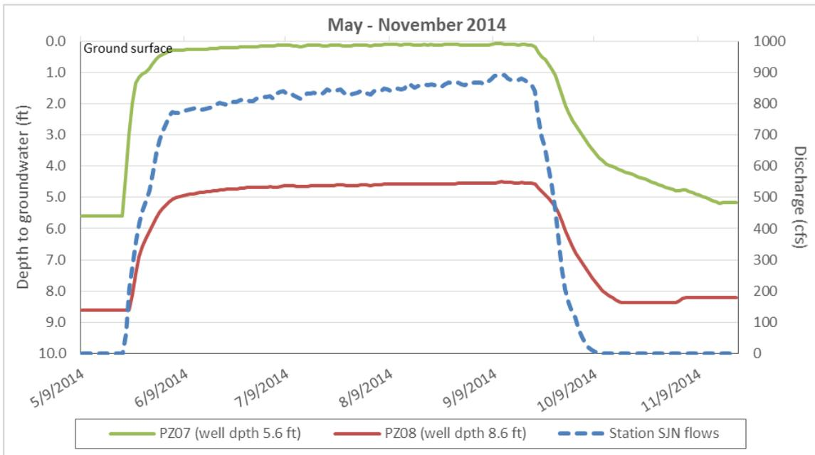
**Figure 14.** Depth to groundwater at wells PZ-7 and -8 and San Joaquin River discharge at gauge SJN from May to November 2014 in Reach 2B.
