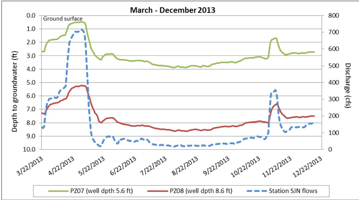
**Figure 13.** Depth to groundwater at wells PZ-7 and -8 and San Joaquin River discharge at gauge SJN from March to December 2013 in Reach 2B.
