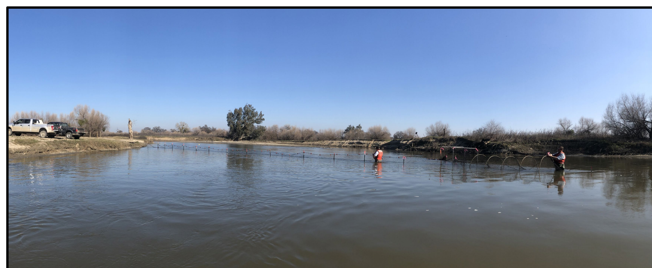
Figure 2. —Fyke net at the Hills Ferry Barrier location in Reach 5 of the San Joaquin River Restoration Area. Note opening(s) and v-shape of wing walls facing downstream.
