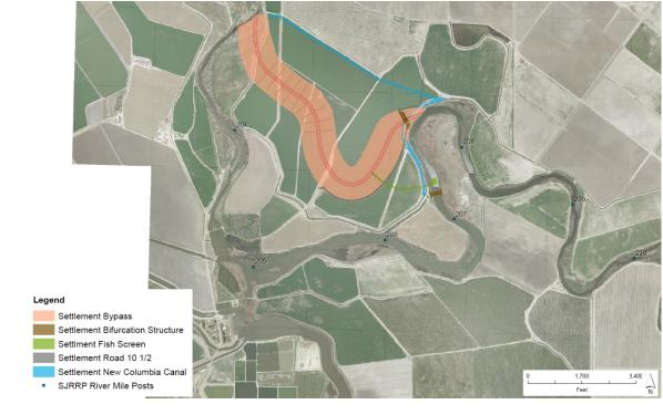
Figure 7-3. Plan View of Settlement Alignment
