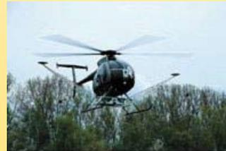
A helicopter equipped with a LIDAR system called FLI-MAP (Fast Laser Imaging - Mapping Airborne Platform) was used to conduct high-resolution surveys, still pictures, and a video record of the levee system.
