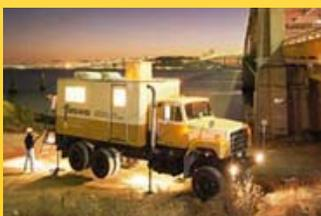
Cone Penetrometer (CPT) rig advancing rod into project levee to estimate soil behavior type.
