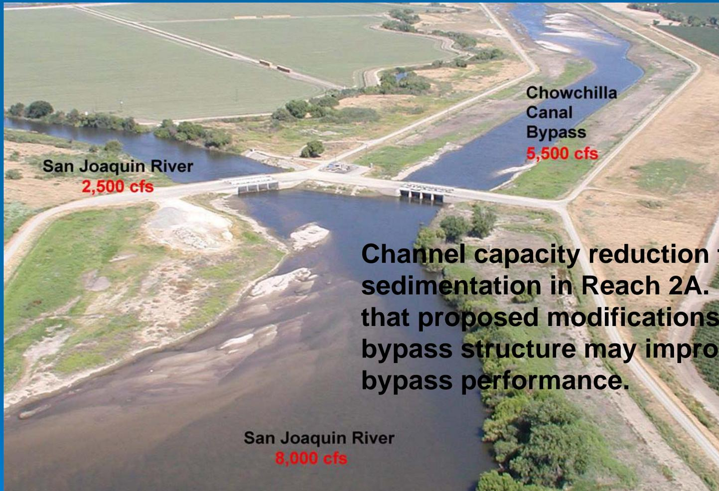
**Channel capacity reduction from sedimentation in Reach 2A. Note that proposed modifications to the bypass structure may improve bypass performance.**
