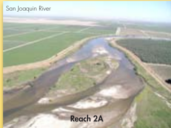
Sedimentation has reduced flow capacity in some reaches.
