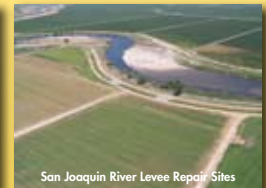
Levees are constructed on unstable foundations consisting of river sediment, mostly sand bars and sand strata. Even low flows can result in numerous sand boils and often levee failure in some reaches.
