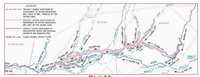
Figure 3-3. Flood Channel Design Flows
