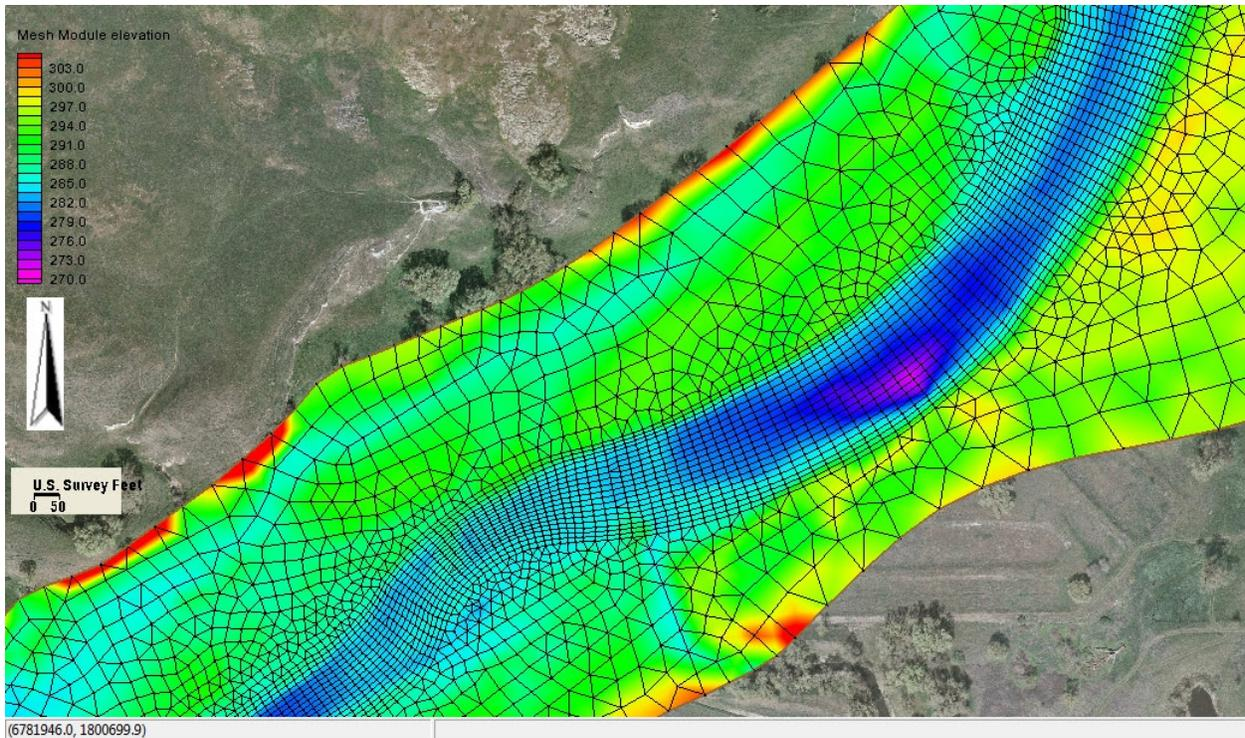
Figure 2. Representative portion (near MP 261.5) of Reach 1A computational mesh developed for SRH-2D hydraulic solver. Bottom elevation (ft, NAVD 88) is mapped to color scale.
