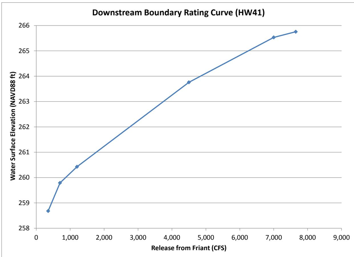
Figure 4. Rating curve used to define downstream boundary condition for Reach 1A\_01 model. Rating data is based on measured water surface elevations at Highway 41 (HW41).
