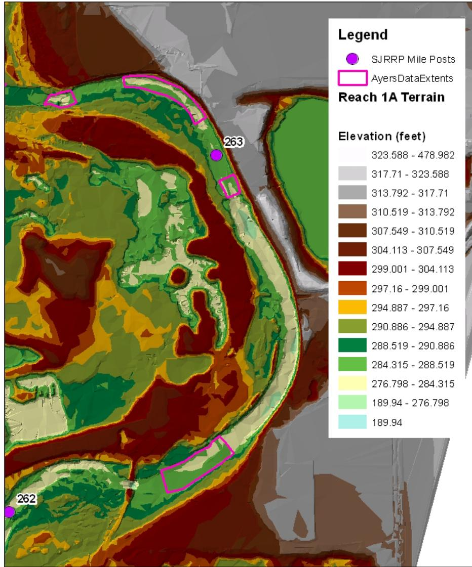
Figure 3. Representative portion of Reach 1A terrain used to populate computational mesh cells. Also shown (purple polygons) are locations where Ayers 1998 data were used in place of 2009 bathymetric data.
