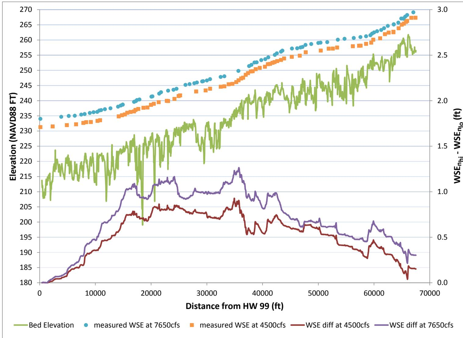
Figure 23. Influence of variation in roughness on predicted water surface elevation along Reach 1A\_02 centerline for floodplain calibration. Primary axis illustrates measured water surface and bed elevation. Secondary axis shows the difference in water surface elevation using the high roughness combination ( $n_{hi} = 50\%$  increase) and the low roughness combination ( $n_{low} = \text{baseline FP } n$ ).
