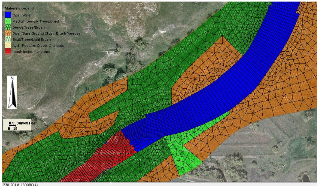
Figure 6. Representative portion of Reach 1A computational mesh near MP 261.5 with land use zones mapped to color scale.
