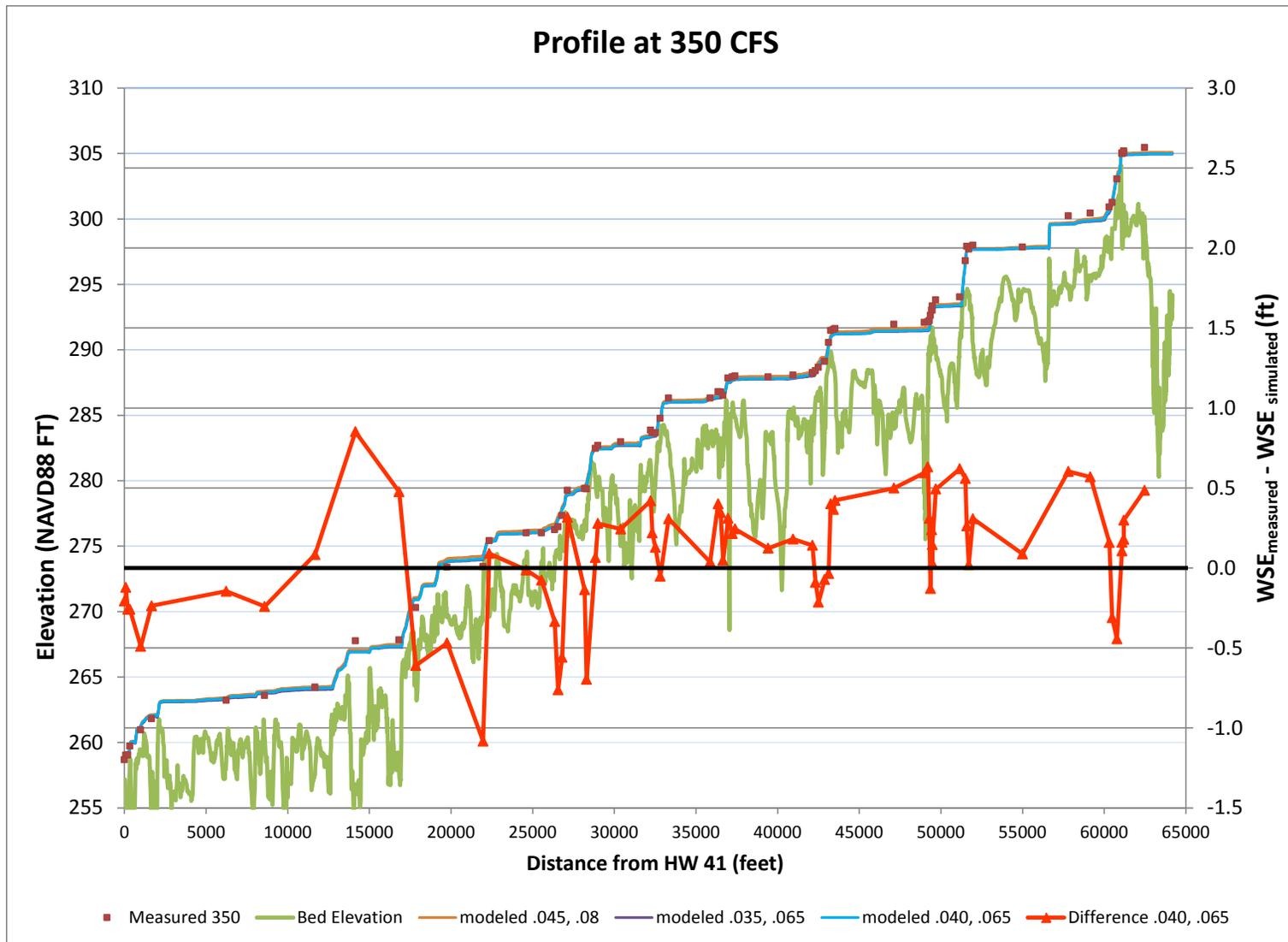
Figure 7. Comparison of measured versus simulated water surface elevation at 350 cfs along the Reach 1A\_01 channel centerline. The secondary axis shows the difference in the measured and simulated (roughness values of .04 and .065) water surface elevation (ft). See Figure 12 for model sensitivity to roughness variation.
