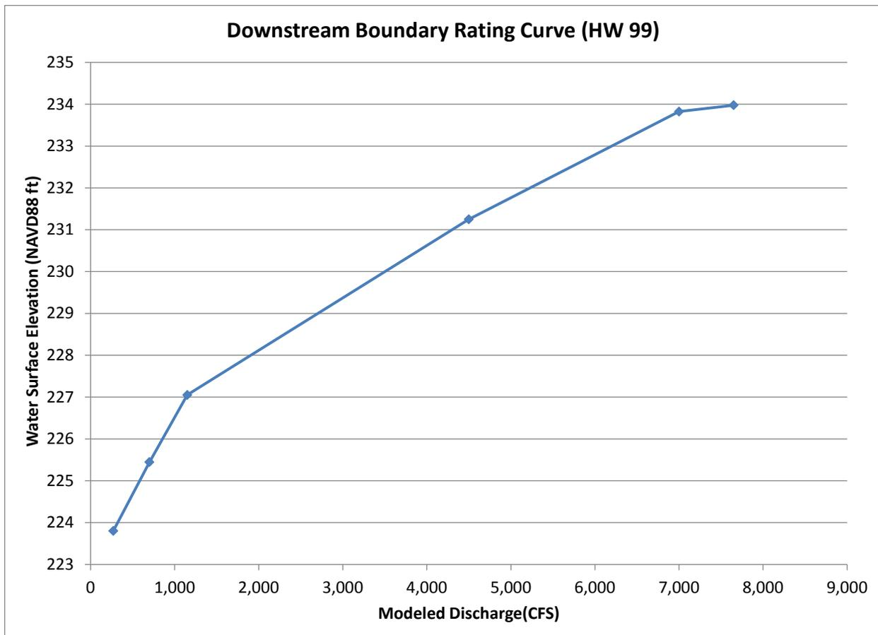
Figure 5. Rating curve used to define downstream boundary condition for Reach 1A\_02 model. Rating data based on measured water surface elevation near Highway 99 (HW99).
