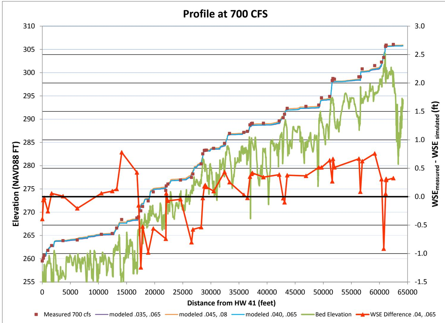
Figure 8. Comparison of measured versus simulated water surface elevation at 700 cfs along the Reach 1A\_01 channel centerline. The secondary axis shows the difference in the measured and simulated (roughness values of .04 and .065) water surface elevation (ft). See Figure 12 for model sensitivity to roughness variation.
