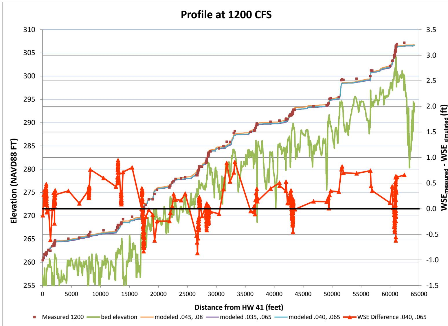
Figure 9. Comparison of measured versus simulated water surface elevation at 1200 cfs along the Reach 1A\_01 channel centerline. Secondary axis shows the difference in the measured and simulated (roughness values of 0.04 and 0.065) water surface elevation (ft). See Figure 12 for model sensitivity to roughness variation.
