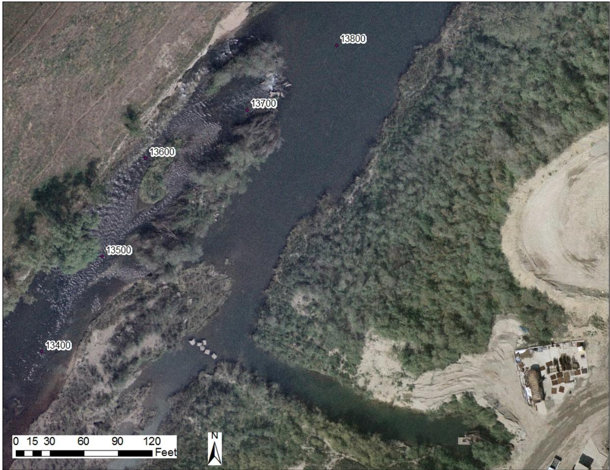
Figure 13. 2007 aerial photo of the location 13,500 feet upstream from HW41, where artificial features are used to create a backwater condition for a gravel mining operation. The topography and mesh do not represent the artificial features or the mid-channel bar well.
