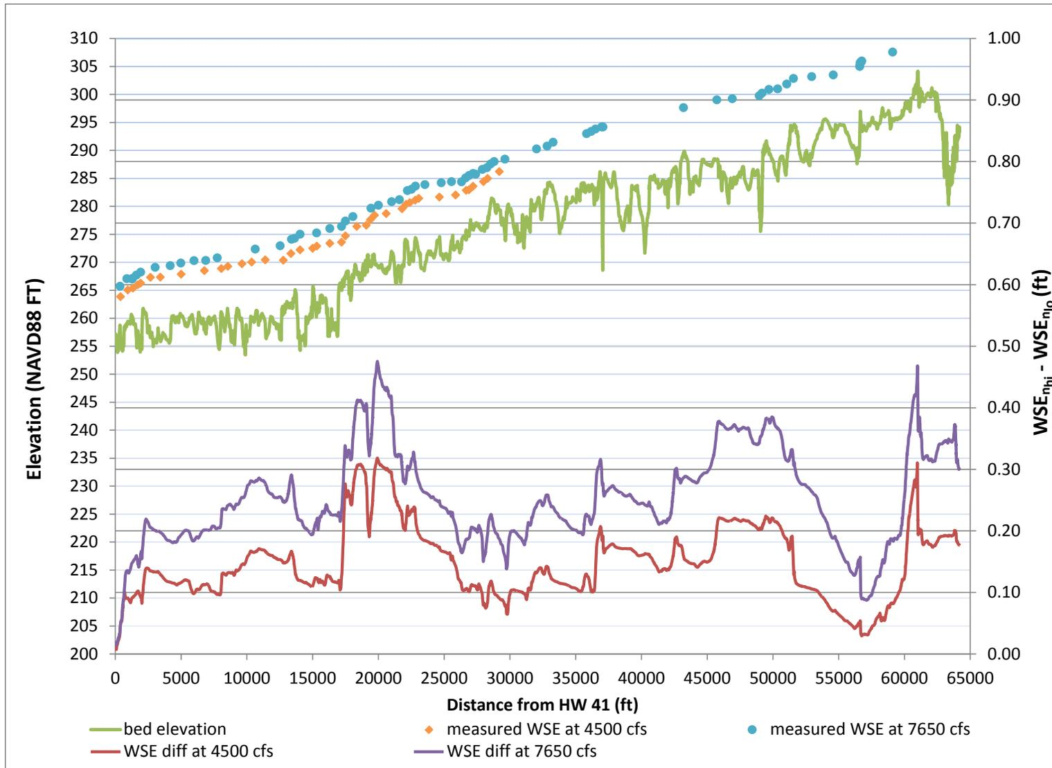
Figure 20. Influence of variation in roughness on predicted water surface elevation along Reach 1A\_01 channel centerline for floodplain calibration. Primary axis illustrates measured water surface and bed elevation. Secondary axis illustrates the difference in water surface elevation using the high roughness combination ( $n_{hi}$  = high FP  $n$ ) and the low roughness combination ( $n_{low}$  = low FP  $n$ ).
