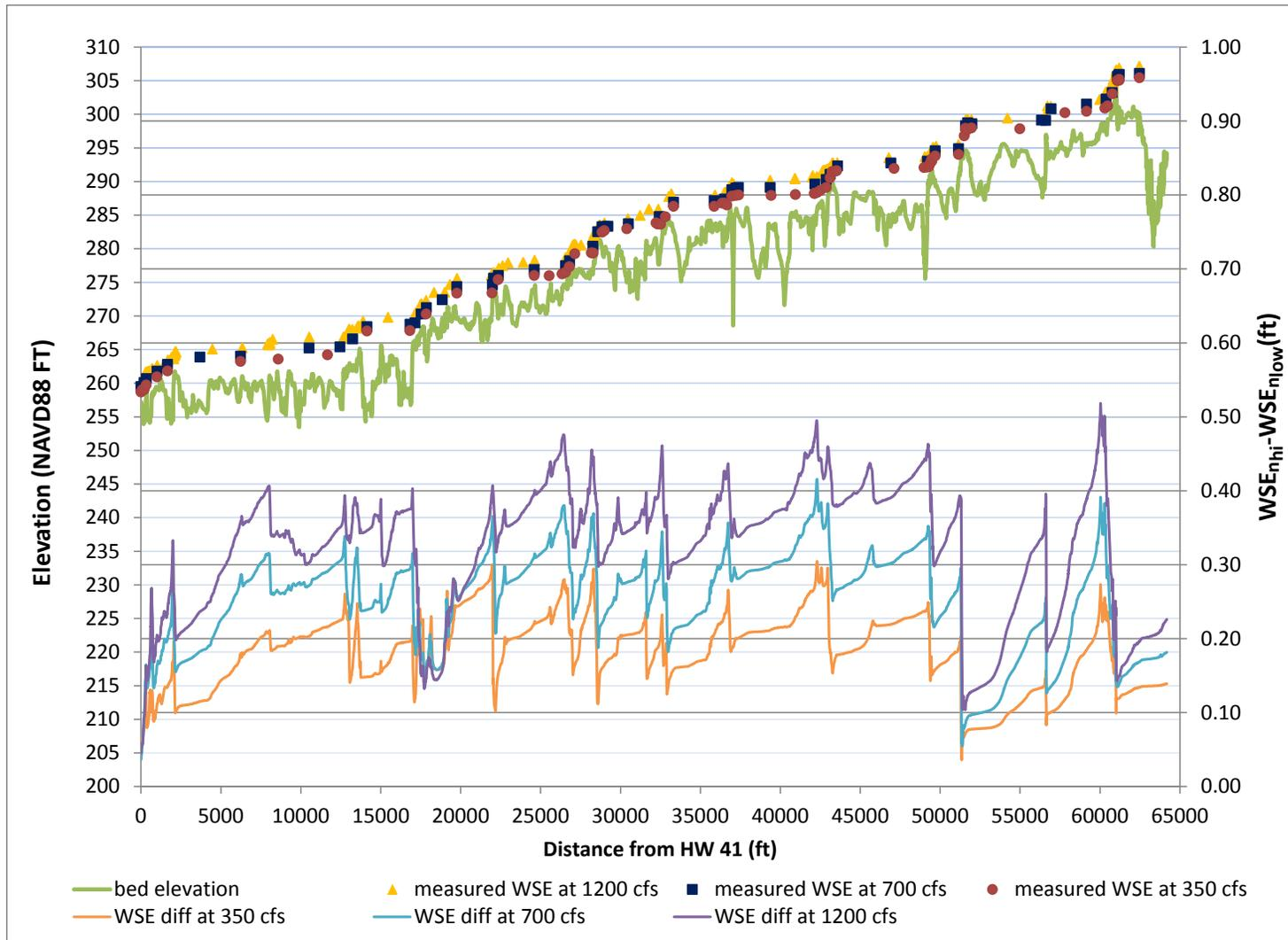
Figure 12. Influence of variation in roughness on predicted water surface elevation along Reach 1A\_01 channel centerline for the in-channel calibration. Primary axis illustrates measured water surface and bed elevation. Secondary axis illustrates the difference in water surface elevation using the high roughness combination ( $n_{hi} = 0.045, 0.08$ ) and the low roughness combination ( $n_{low} = 0.035, 0.065$ ).
