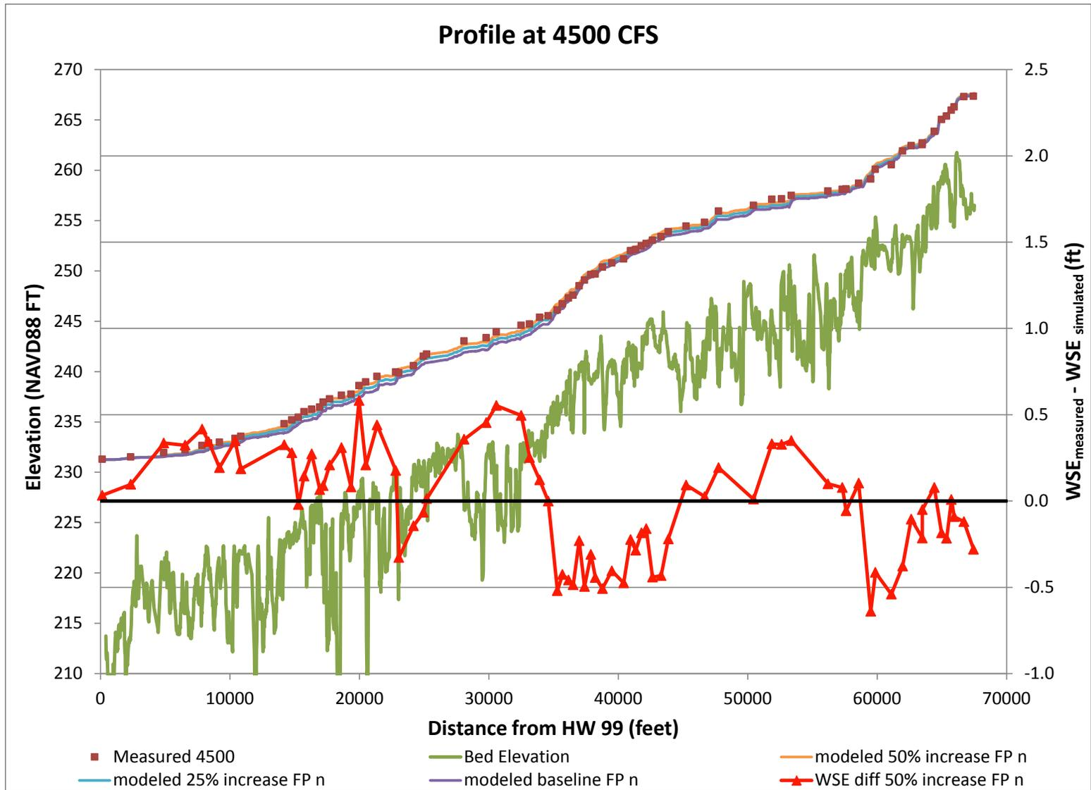
Figure 21. Comparison of measured versus simulated water surface elevation at 4500 cfs along the channel centerline in Reach 1A\_02. Secondary axis shows the difference in measured and simulated water surface elevation (ft) for roughness values increase 50% above baseline values. See Figure 23 for model sensitivity to roughness variation.
