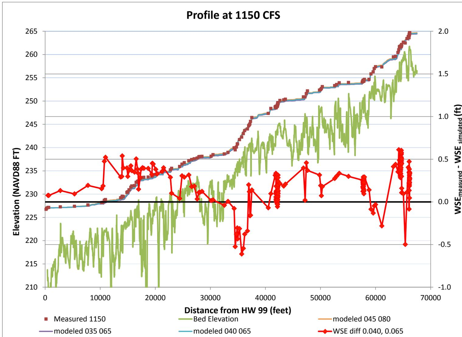
Figure 16. Comparison of measured versus simulated water surface elevation at 1150 cfs along the Reach 1A\_02 channel centerline. The secondary axis shows the difference in the measured and simulated (roughness values of .04 and .065) water surface elevation (ft). See Figure 17 for model sensitivity to roughness variation.
