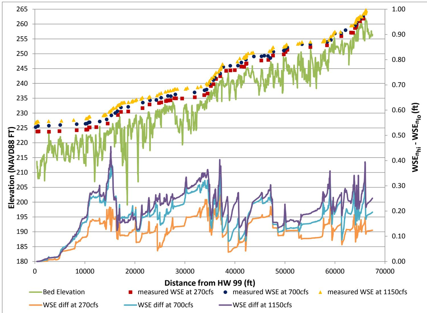
Figure 17. Influence of variation in roughness on predicted water surface elevation along Reach 1A\_02 channel centerline for the in-channel calibration. Primary axis illustrates measured water surface and bed elevation. Secondary axis illustrates the difference in water surface elevation using the high roughness combination ( $n_{hi} = .045, .08$ ) and the low roughness combination ( $n_{low} = .035, .065$ ).
