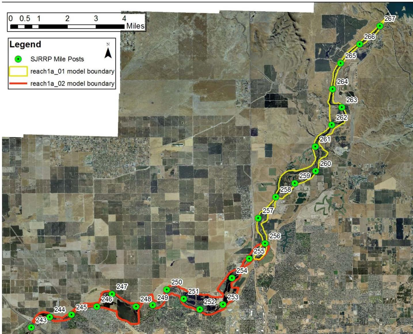
Figure 1. Map of Reach 1 of the San Joaquin River showing the two model boundaries used in this effort. Reach 1A\_01 extends from Friant Dam to HW 41, and Reach 1A\_02 extends from HW41 to HW99.
