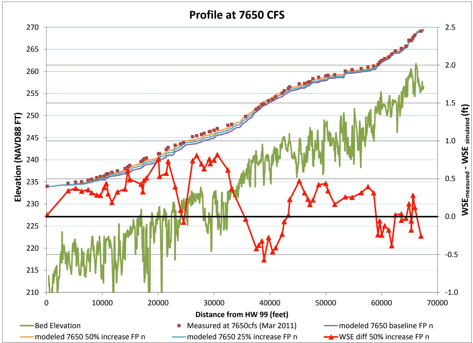
Figure 22. Comparison of measured versus simulated water surface elevation at 7650 cfs along the channel centerline in Reach 1A\_02. Secondary axis shows the difference in measured and simulated water surface elevation (ft) for roughness values increased 50% above baseline values. See Figure 23 for model sensitivity to roughness variation.
