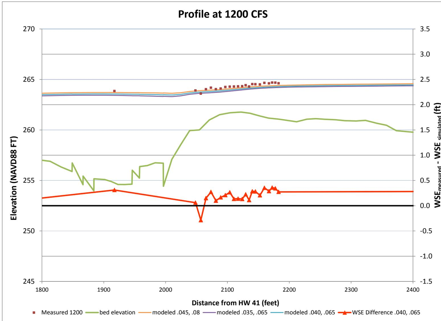
Figure 10. Comparison of measured versus simulated water surface elevation at 1200 cfs along a riffle near MP 260.7. Secondary axis shows the difference in the measured and simulated (roughness values of 0.04 and 0.065) water surface elevation (ft).
