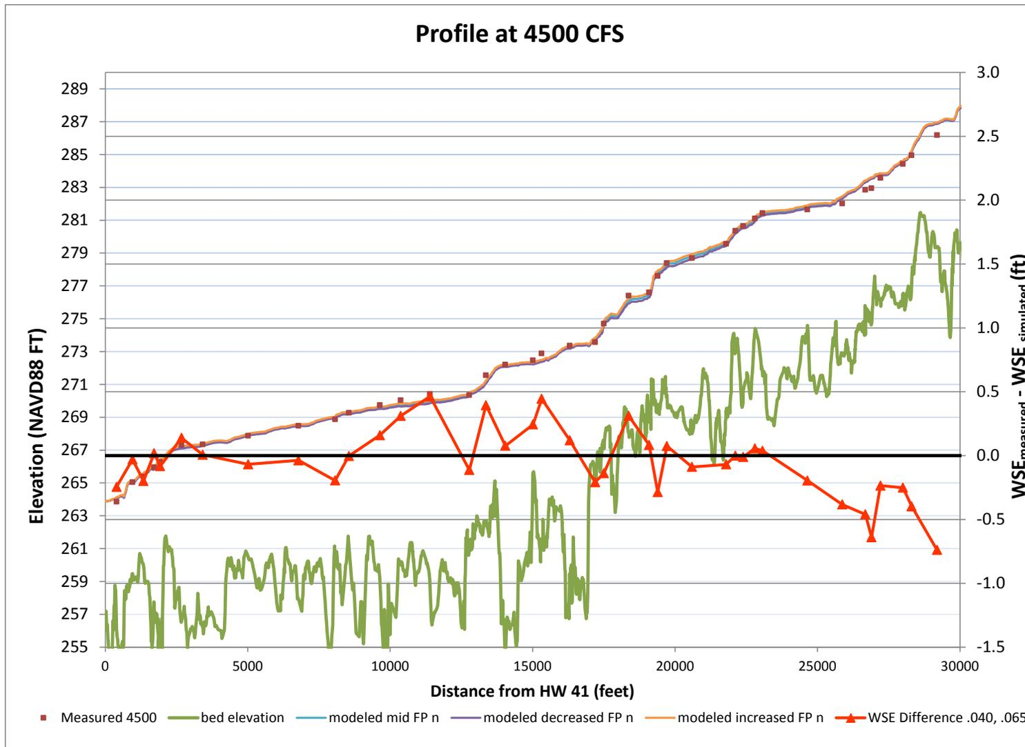
Figure 18. Comparison of measured versus simulated water surface elevation at 4500 cfs along the channel centerline in Reach 1A\_01. Secondary axis shows the difference in measured and simulated (roughness values of .04 and .065) water surface elevation (ft). See Figure 20 for model sensitivity to roughness variation.
