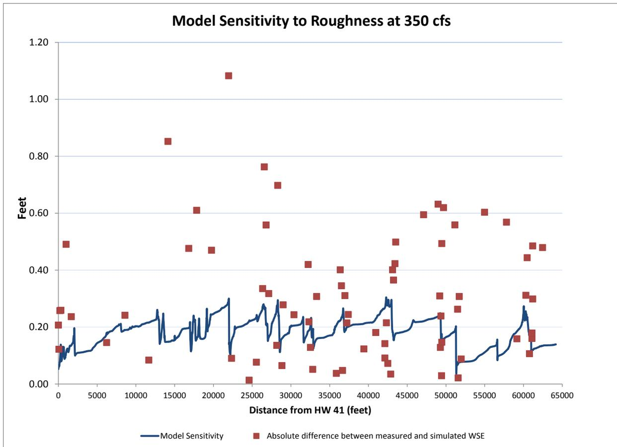
Figure 25. Comparison of model sensitivity to roughness and the absolute difference in measured and simulated water surface. Model sensitivity represents the difference in the simulated water surface using the highest roughness combination and the simulated water surface using the lowest roughness combination.
