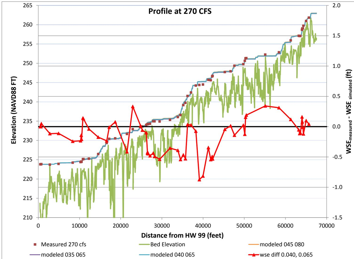
Figure 14. Comparison of measured versus simulated water surface elevation at 270 cfs along the Reach 1A\_02 channel centerline. The secondary axis shows the difference in the measured and simulated (roughness values of .04 and .065) water surface elevation (ft). See Figure 17 for model sensitivity to roughness variation.
