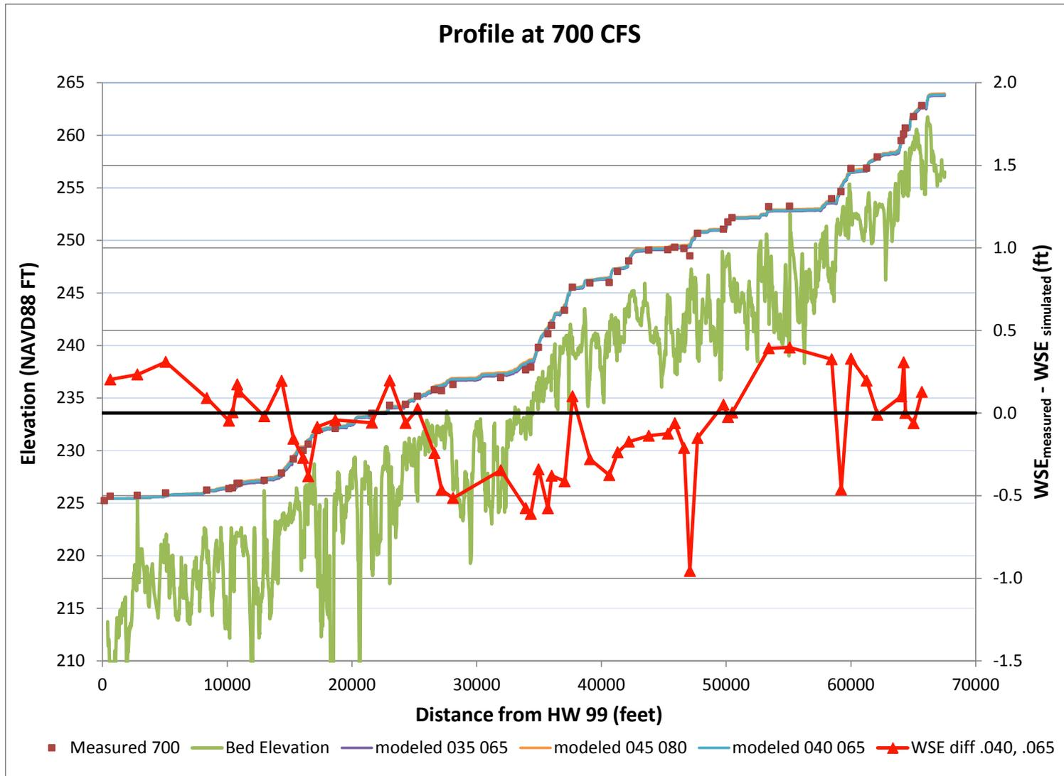
Figure 15. Comparison of measured versus simulated water surface elevation at 700 cfs along the Reach 1A\_02 channel centerline. The secondary axis shows the difference in the measured and simulated (roughness values of .04 and .065) water surface elevation (ft). See Figure 17 for model sensitivity to roughness variation.
