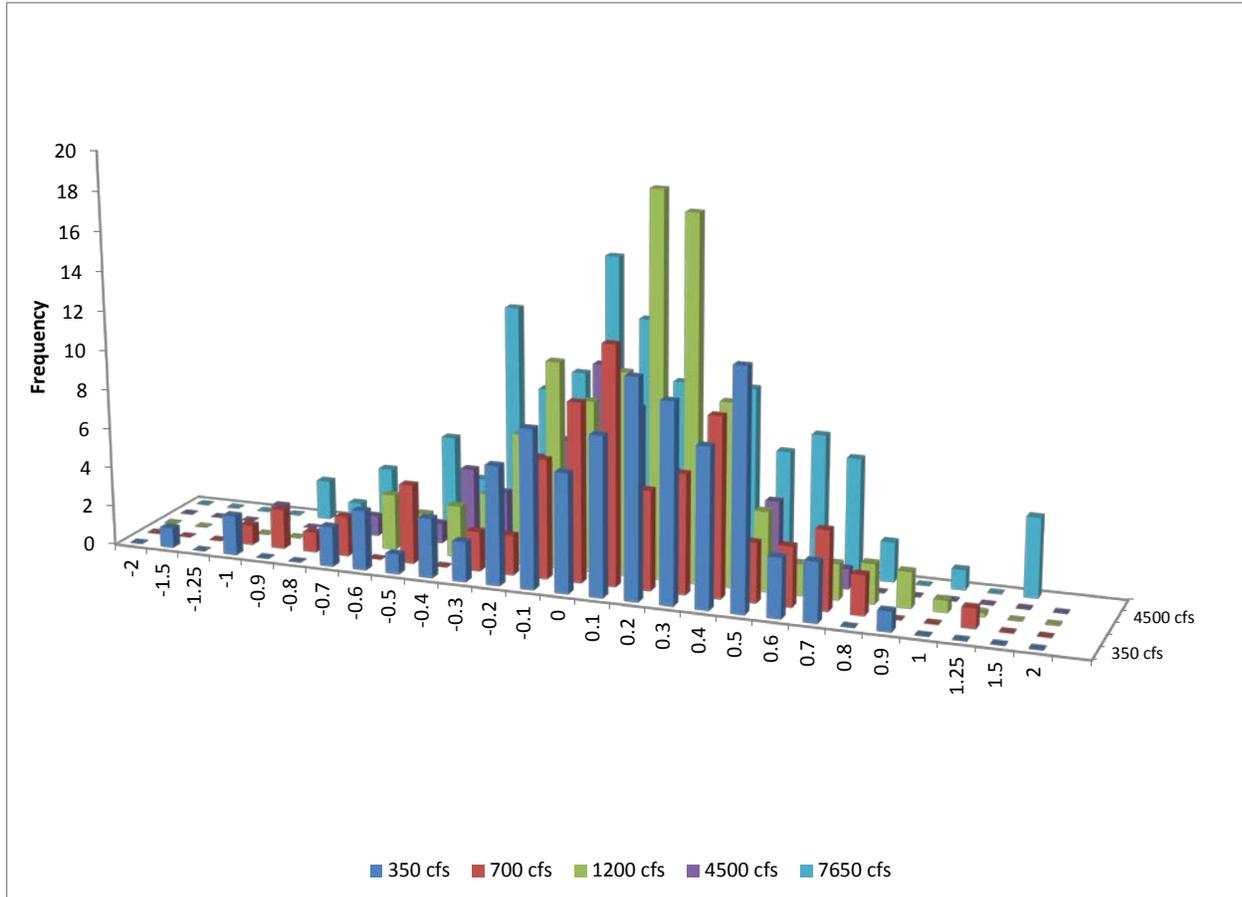
Figure 24. Histogram of point differences between measured and simulated water surface elevations (ft) at each discharge. A negative value indicates that the simulated value was higher than the measured value. Because 1200 cfs had 5 times more measured points than other flows, each frequency value was divided by 5.
