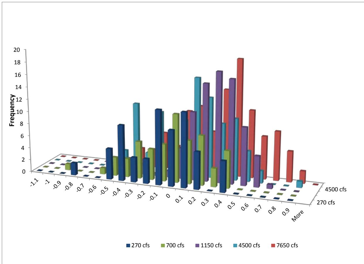
Figure 26. Histogram of point differences between measured and simulated water surface elevation (ft) at each discharge. A negative value indicates that the simulated value was higher than the measured value. Because 1150 cfs had 2.5-3 times more measured points than other discharges, each frequency value was divided by 3.
