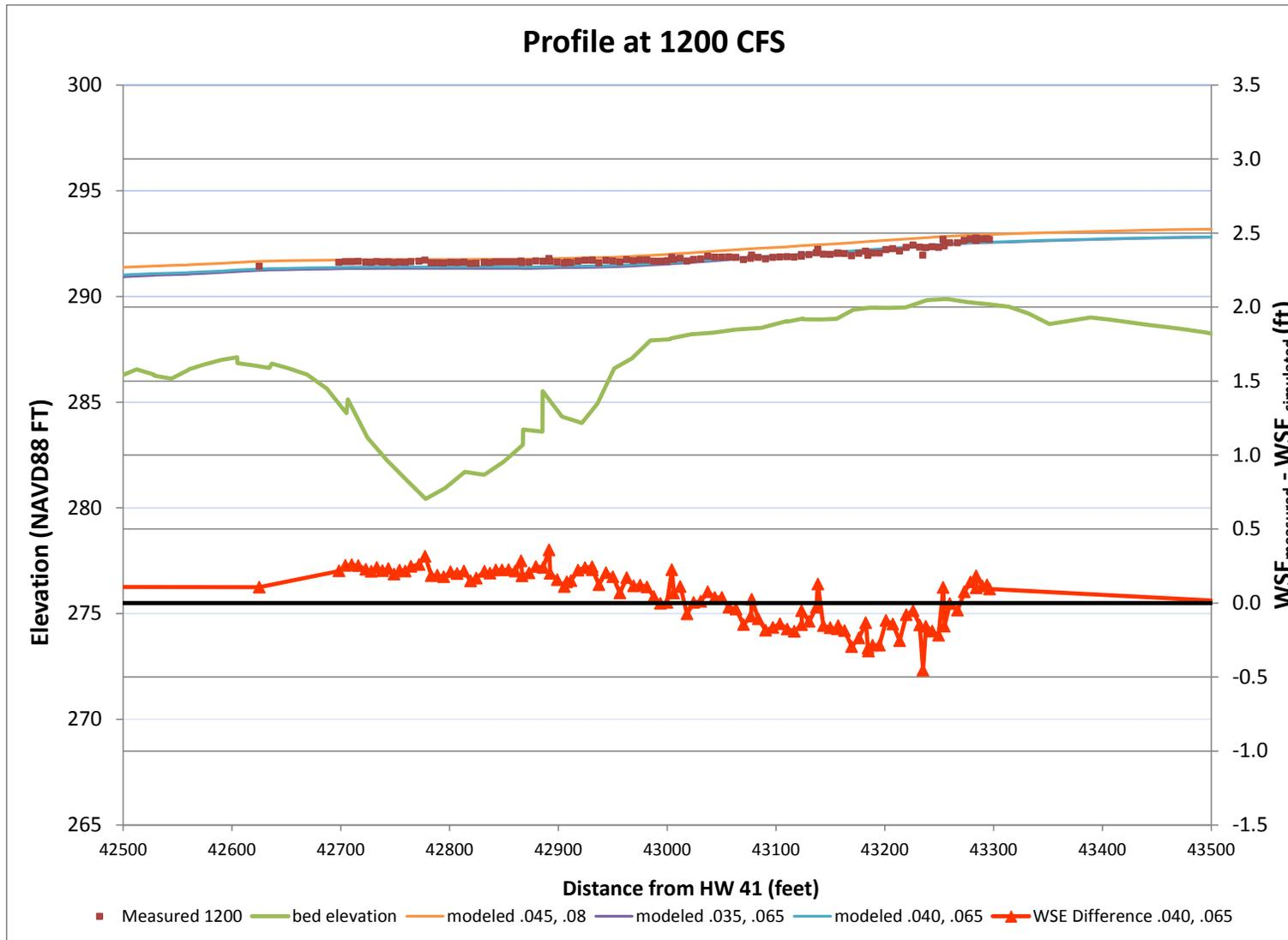
Figure 11. Comparison of measured versus simulated water surface elevation at 1200 cfs along a riffle near MP 263.3. Secondary axis shows the difference in the measured and simulated (roughness values of 0.04 and 0.065) water surface elevation (ft).
