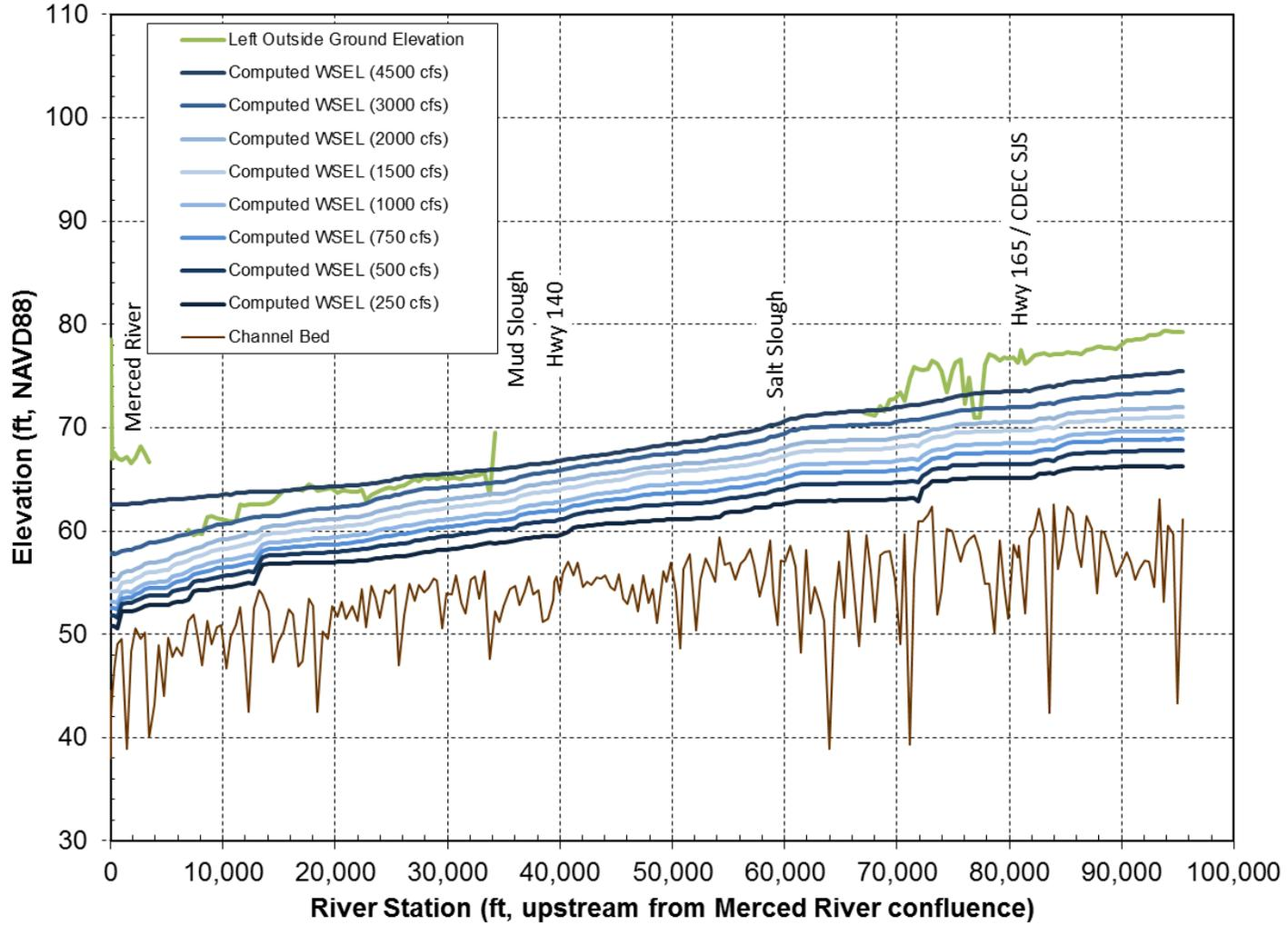
Figure 22. Comparison of outside ground elevation with computed water-surface elevations along left levee in Reach 5.
