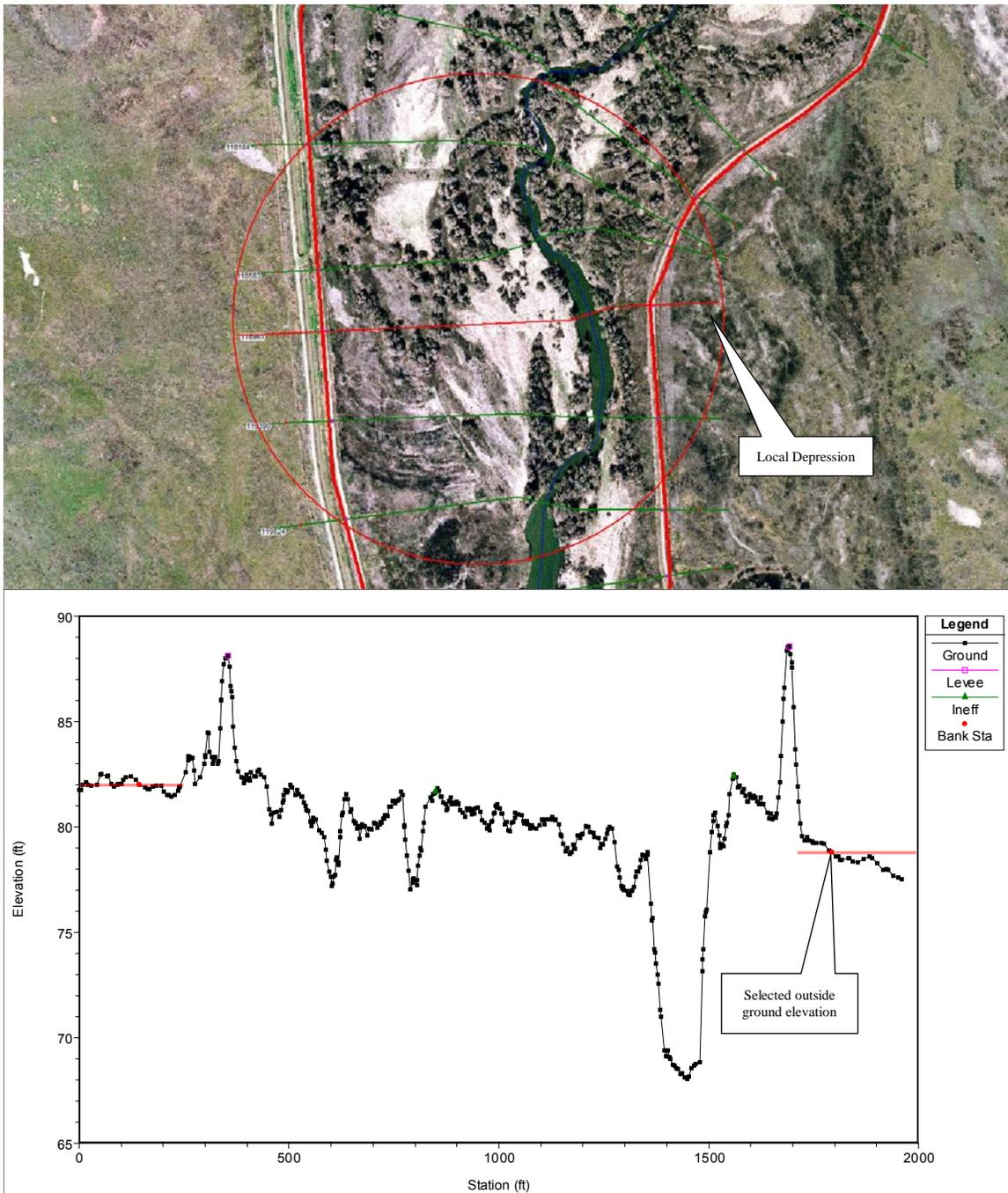
Figure A.2: Reach 4B2 – Plan and profile view of XS 118961. The right overbank slopes away from the levee into an oxbow.
