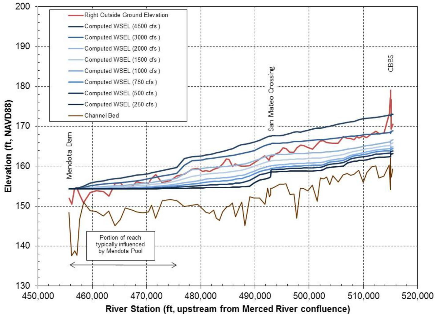
Figure 6. Comparison of outside ground elevation with computed water-surface elevations along right levee in Reach 2B.
