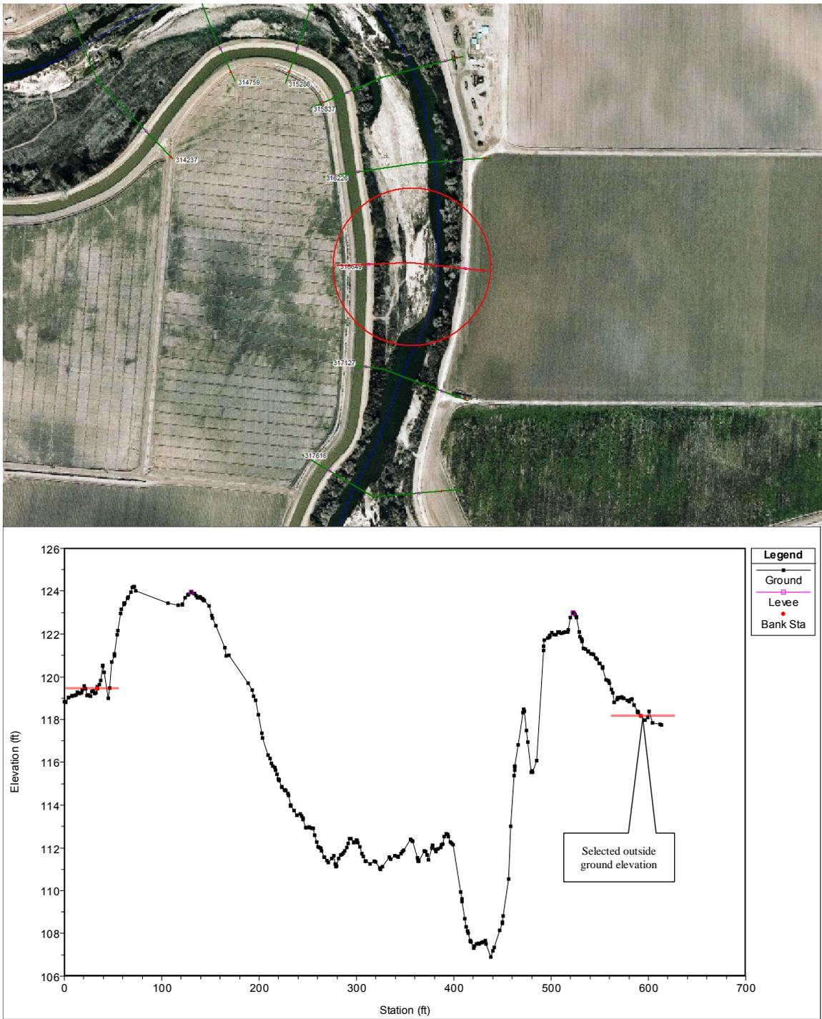
Figure A.4: Reach 4A – Plan and profile view of XS 316649. The right overbank slopes away from the levee.
