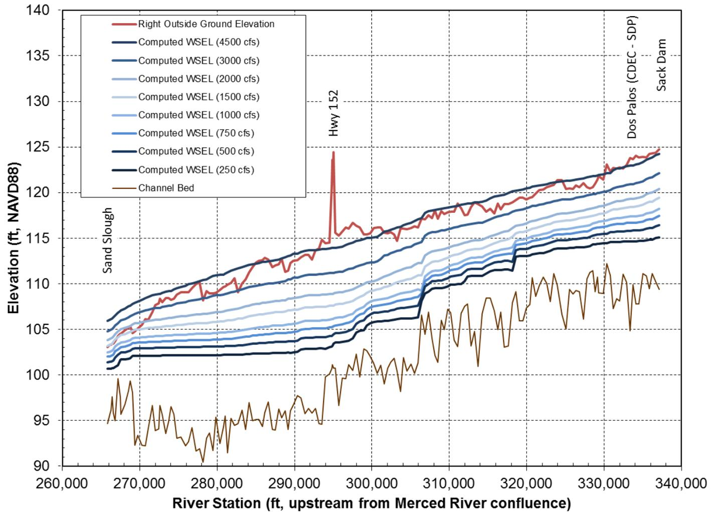
Figure 13. Comparison of outside ground elevation with computed water-surface elevations along right levee in Reach 4A.
