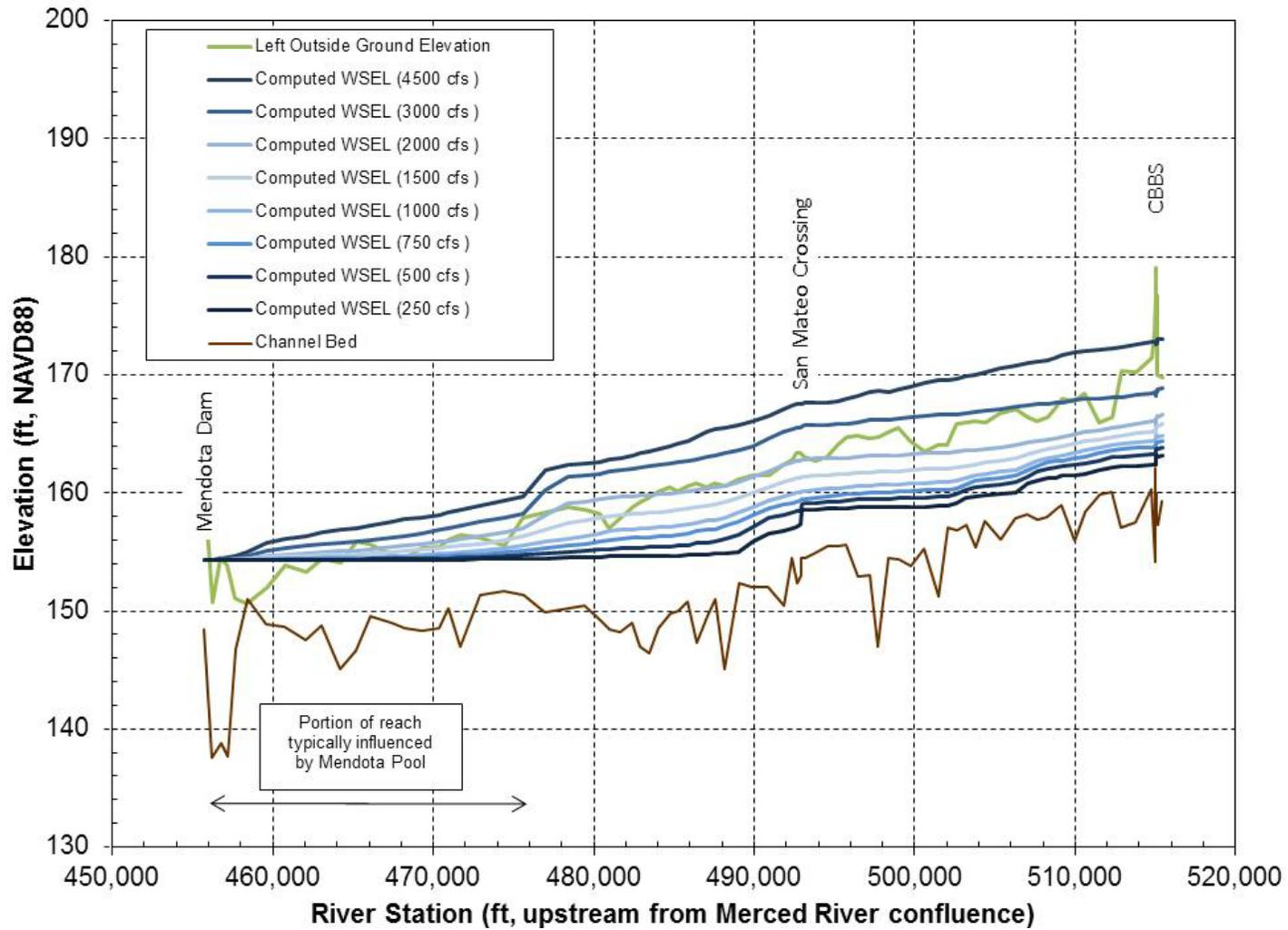
Figure 7. Comparison of outside ground elevation with computed water-surface elevations along left levee in Reach 2B.
