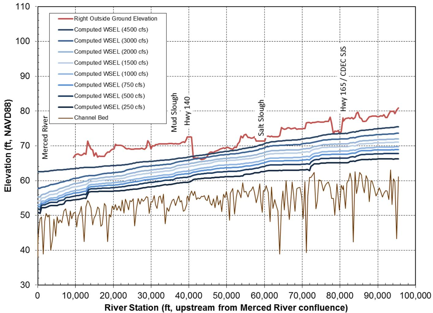
Figure 21. Comparison of outside ground elevation with computed water-surface elevations along right levee in Reach 5.
