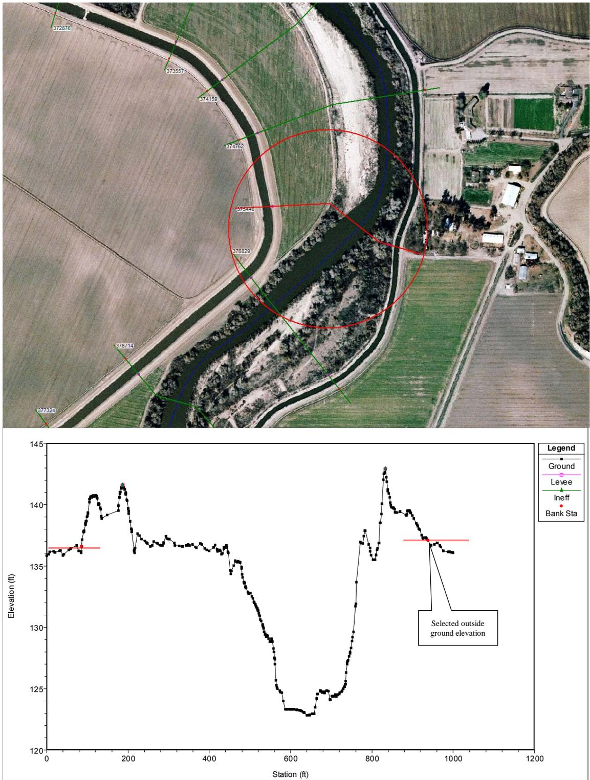
Figure A.6: Reach 3 – Plan and profile view of XS 375446. The right overbank slopes away from the levee.
