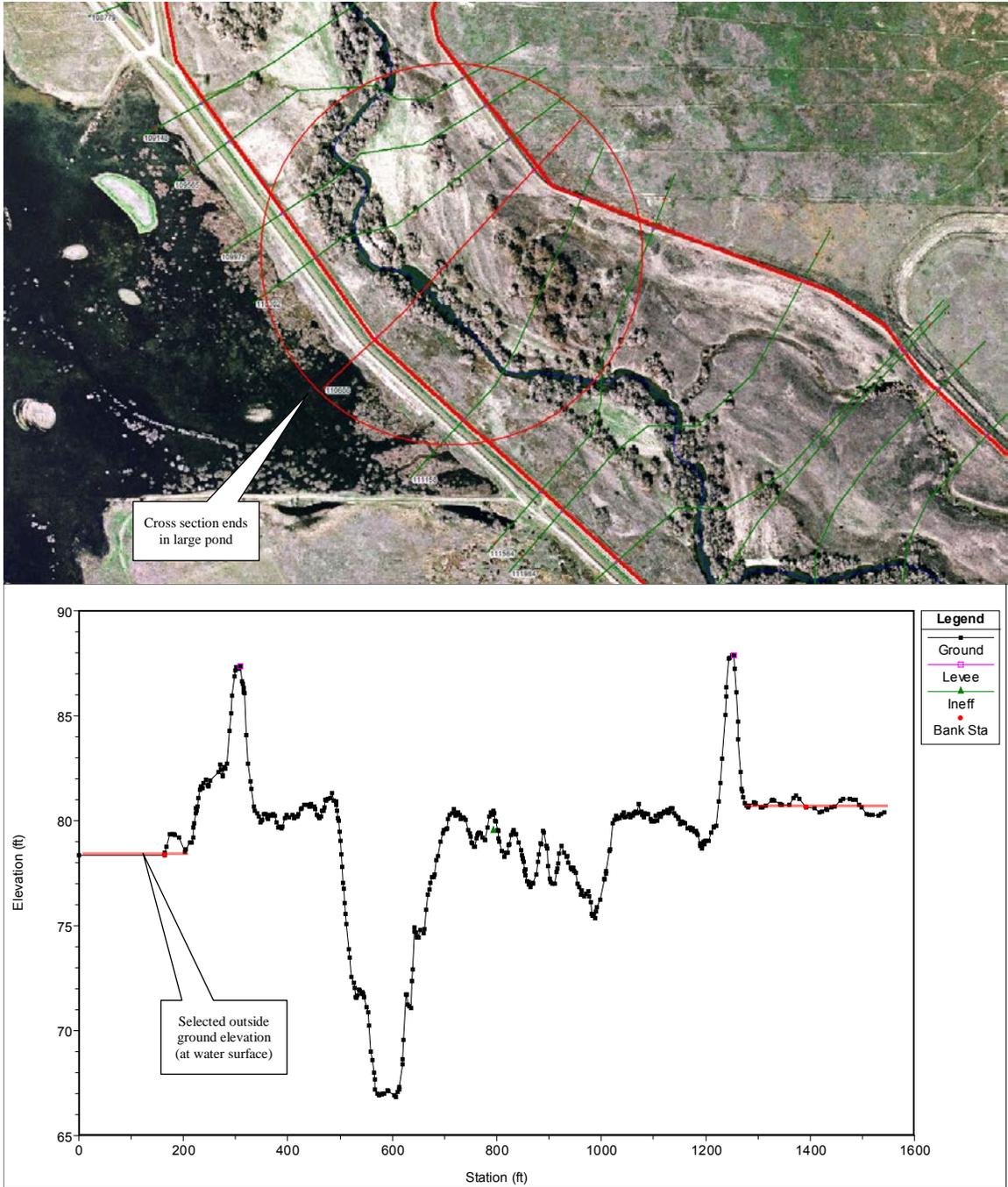
Figure A.1: Reach 4B2 – Plan and profile view of XS 110688. The left side of the cross section terminates in a pond immediately adjacent to the levee.
