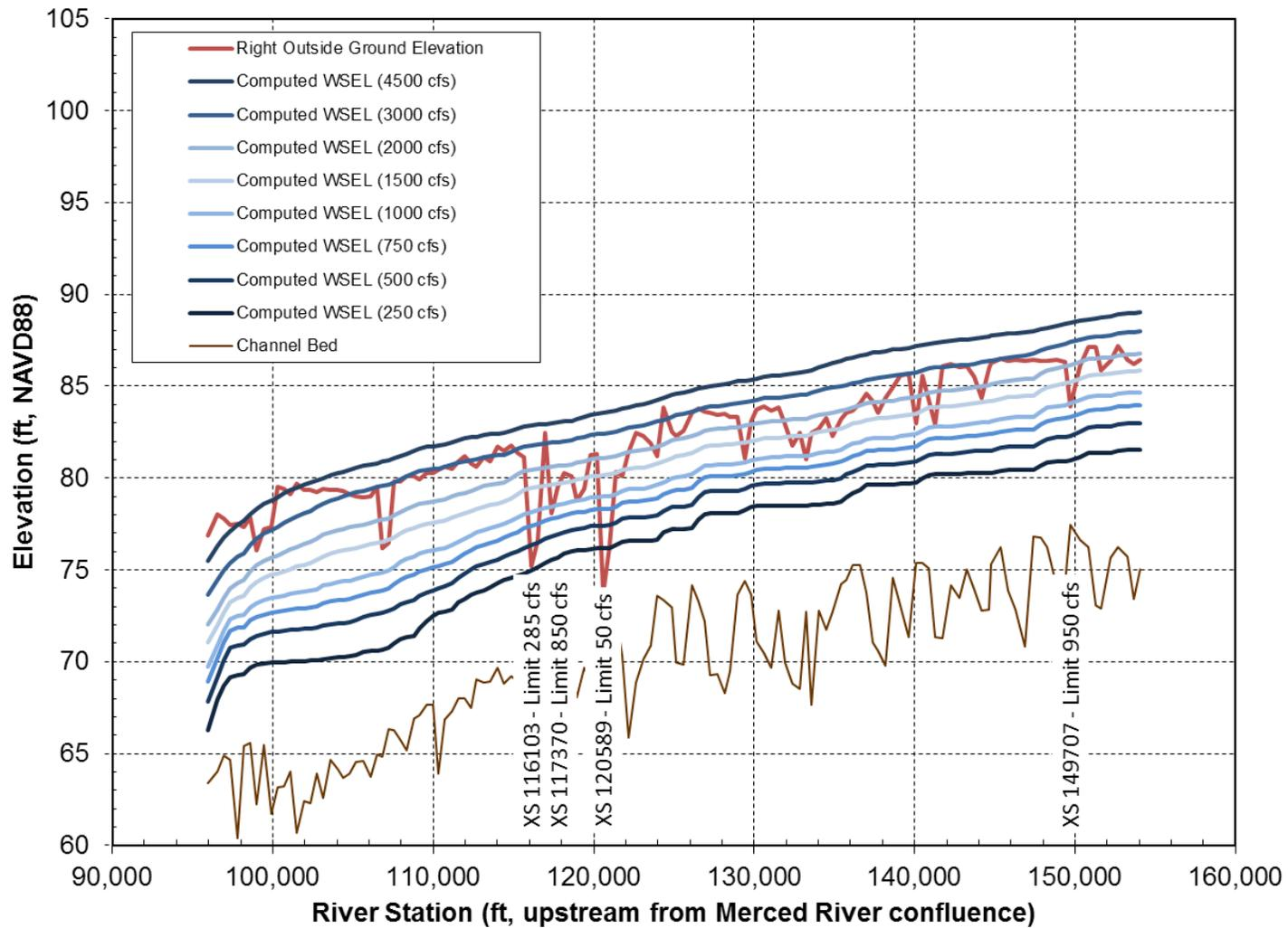
Figure 17. Comparison of outside ground elevation with computed water-surface elevations along right levee in Reach 4B2.
