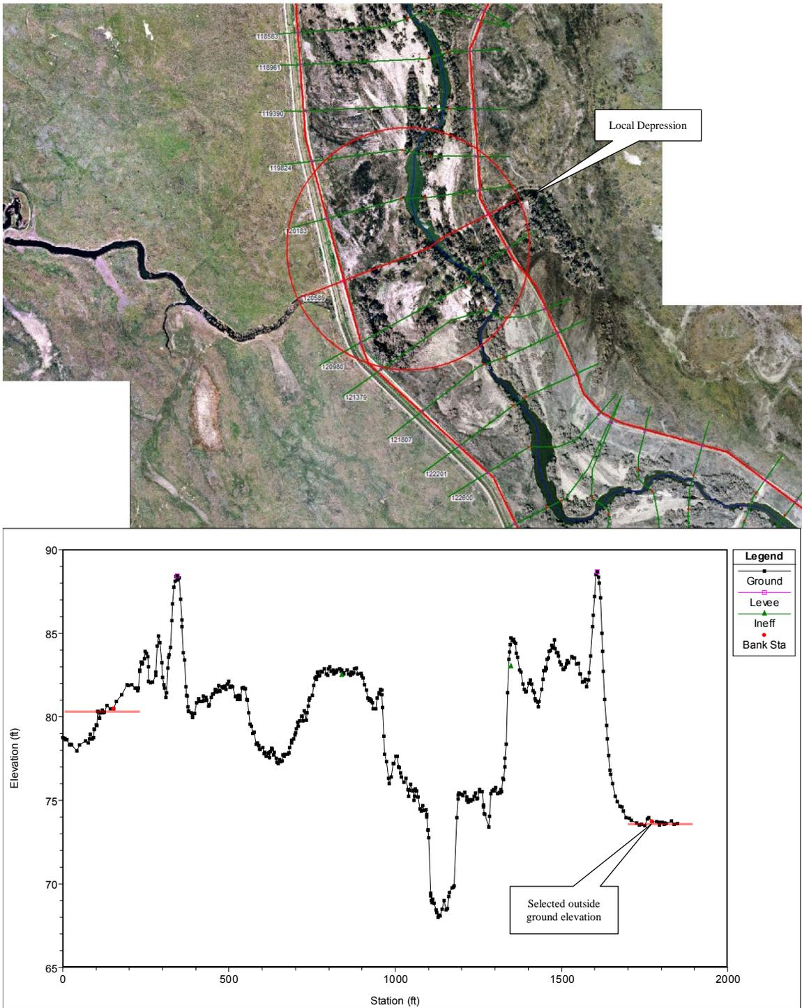
Figure A.3: Reach 4B2 – Plan and profile view of XS 120589. The right overbank ends in a local depression.
