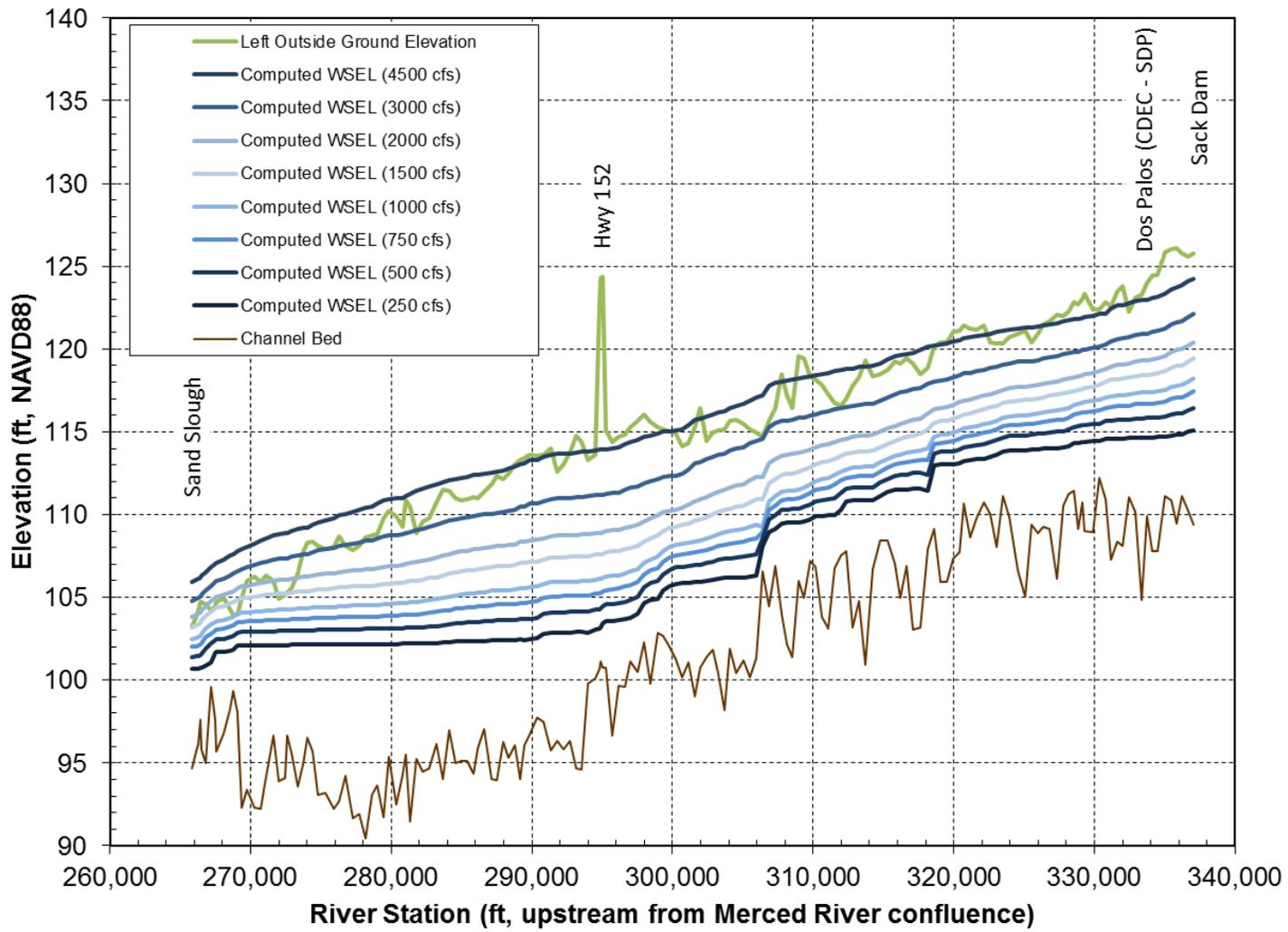
Figure 14. Comparison of outside ground elevation with computed water-surface elevations along left levee in Reach 4A.
