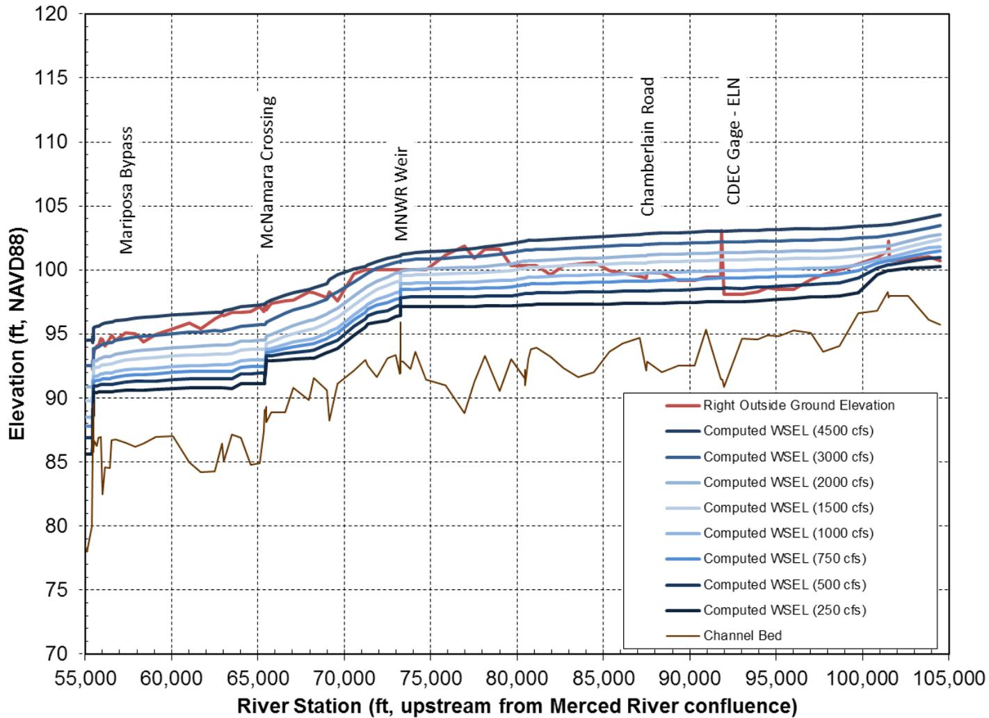
Figure 25. Comparison of outside ground elevation with computed water-surface elevations along right levee in Middle Eastside Bypass.
