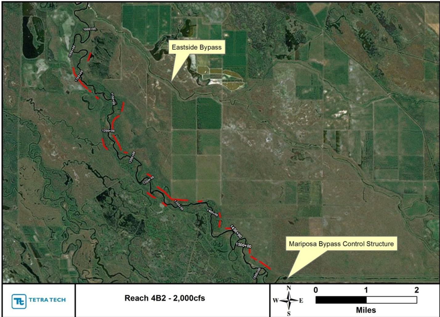
Figure 19. Portions of levee in Reach 4B2 where the 2,000-cfs water-surface elevation is above the existing outside ground elevation.
