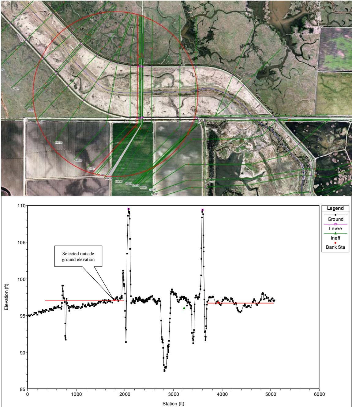
Figure A.7: Middle ESB – Plan and profile view of XS 65344. The left overbank slopes away from levee.
