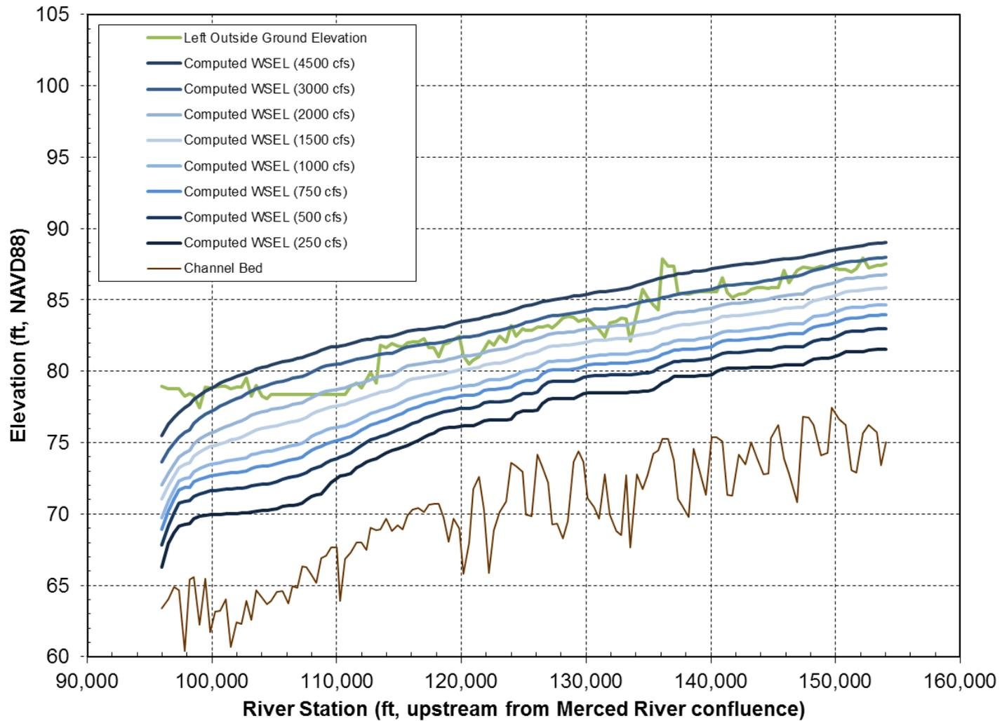
Figure 18. Comparison of outside ground elevation with computed water-surface elevations along left levee in Reach 4B2.
