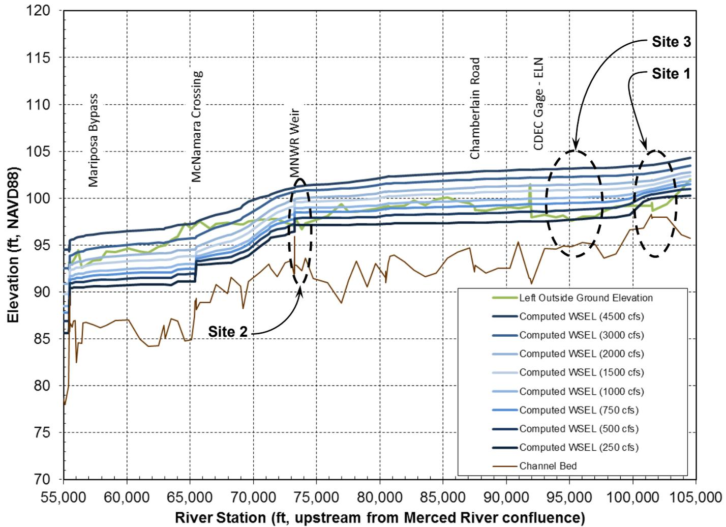
Figure 26. Comparison of outside ground elevation with computed water-surface elevations along left levee in Middle Eastside Bypass as well as identification of the three critical sites along the left levee.
