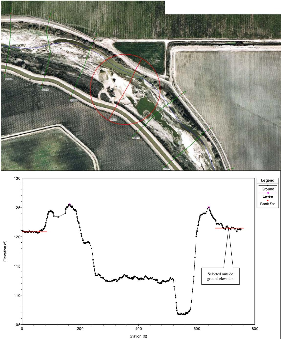
Figure A.5: Reach 4A – Plan and profile view of XS 324528. The right overbank slopes gradually away from the levee.
