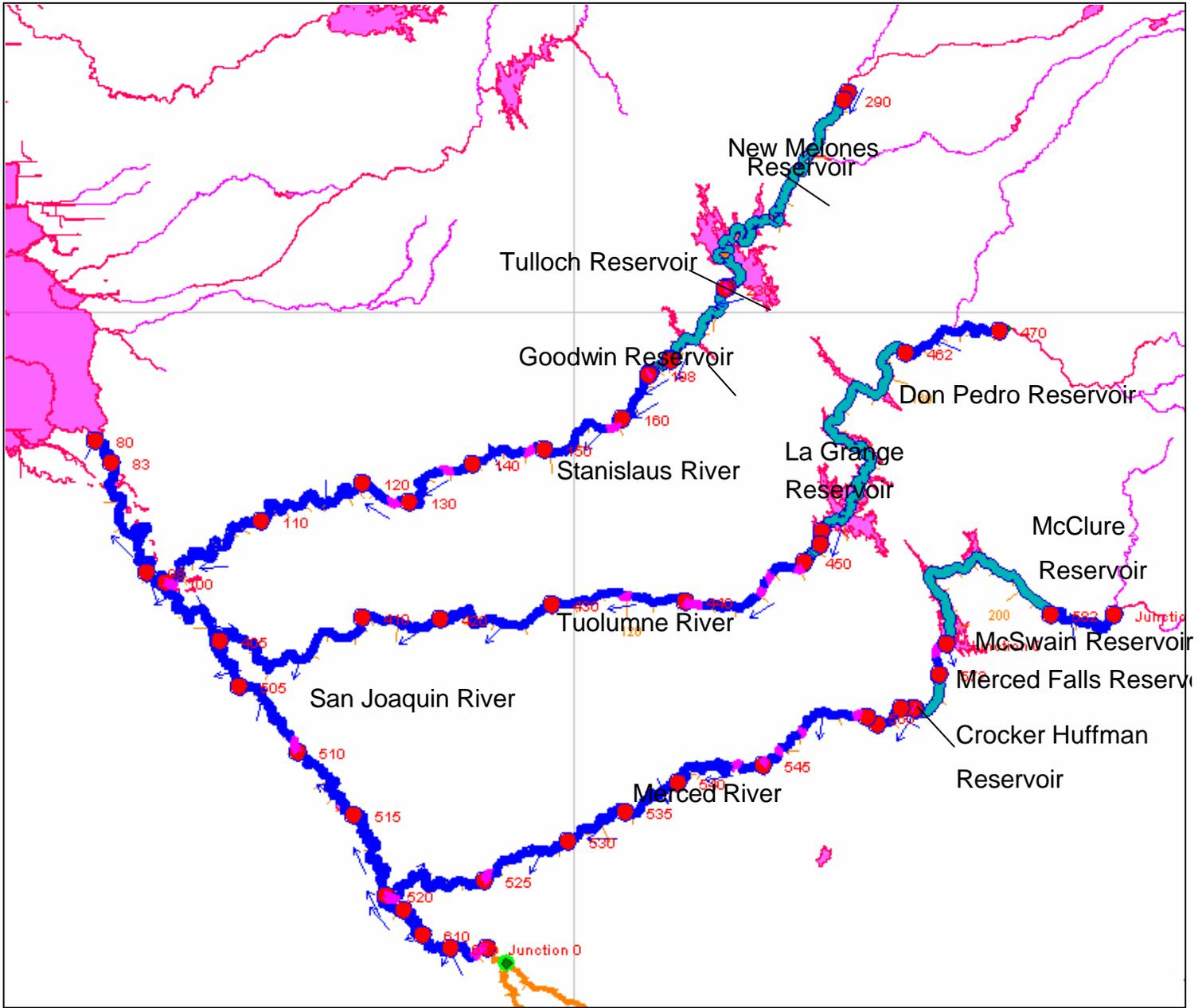
Figure 1-1 Schematic of HEC-5 model of the Stanislaus/Tuolumne/Merced River system
