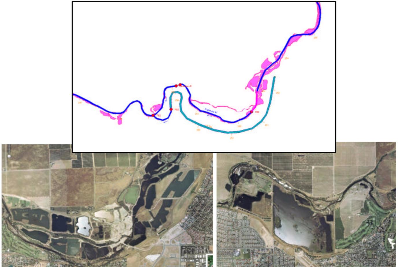
Figure 3-9 Model representation of interflow between river and gravel pits/alluvial deposits, and aerial photos showing gravel pits
