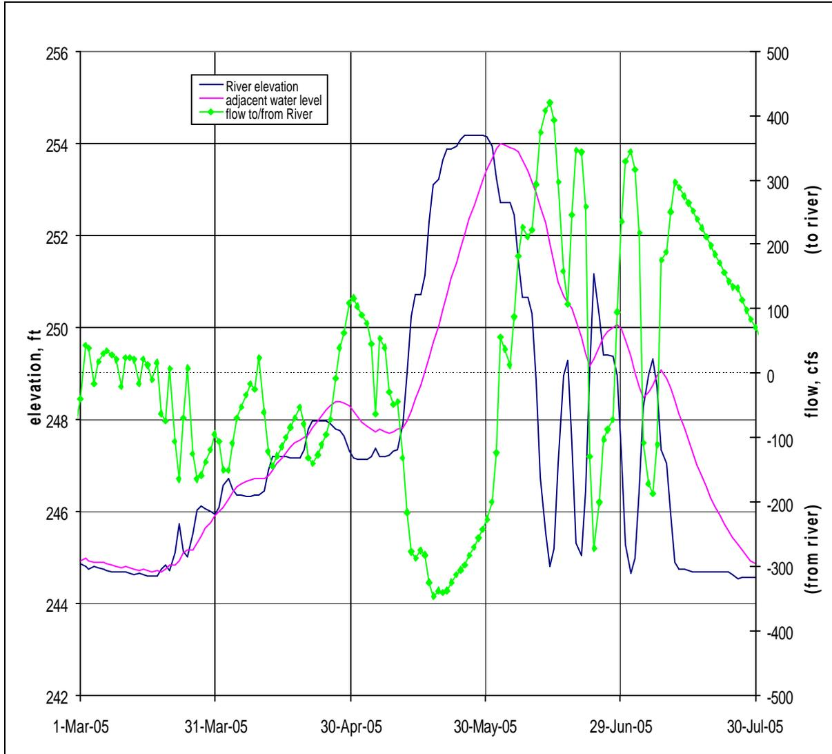
Figure 3-10 Hypothetical interflow between river and gravel pits/alluvial deposits as a function of river elevation
