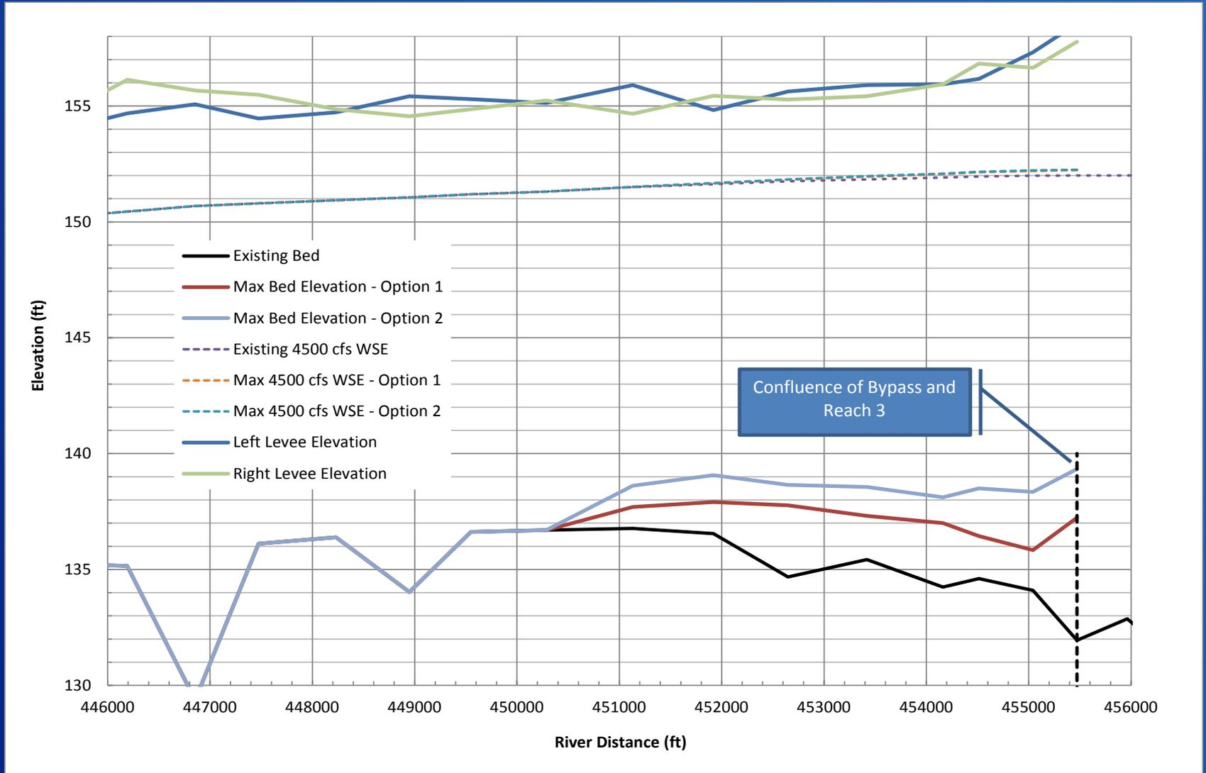
**Simulations do not indicate that 4500 cfs will encroach into the 3 feet of freeboard**
