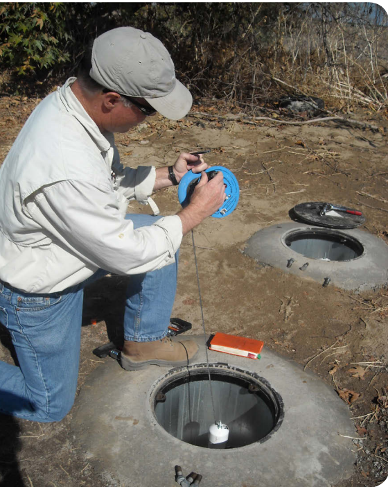
Measurements are taken regularly at groundwater monitoring wells
