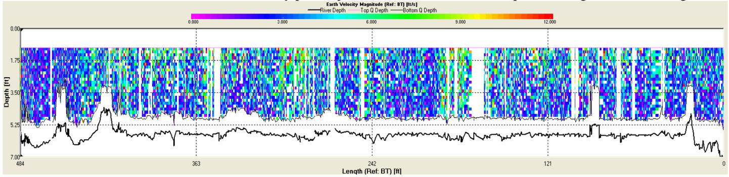
ESBS@MB 1-001. ADCP cross section velocity profile just downstream structure during flow monitoring
