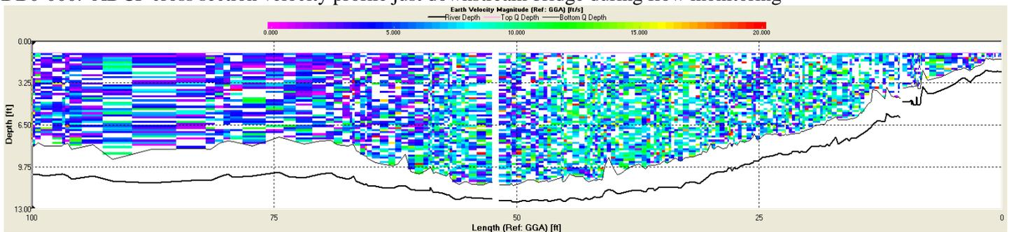
DB0-002. ADCP cross section velocity profile just upstream the bridge in bay 3
