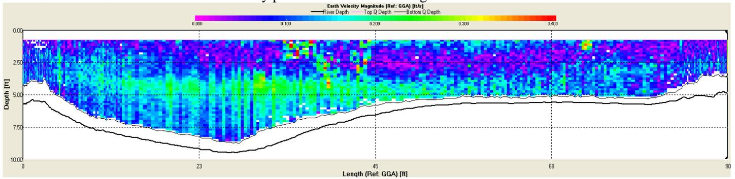
BD1&2-1-004. ADCP cross section velocity profile just downstream beaver dam 1 during flow monitoring
