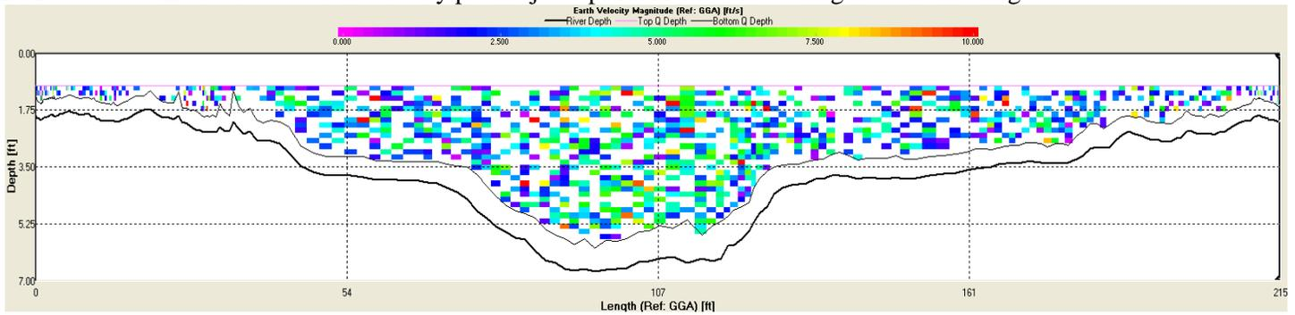
DMC 1-000. ADCP cross section velocity profile on portion of the road during flow monitoring
