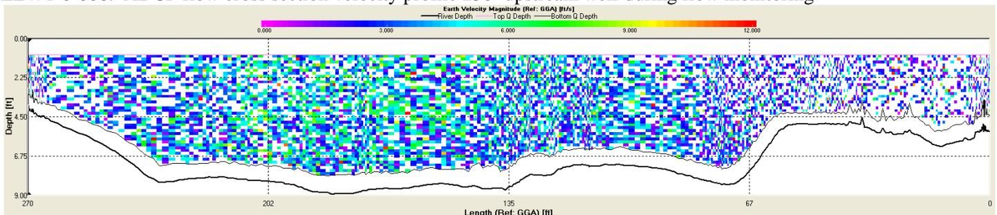
LLW1-1-000. ADCP cross section velocity profile just upstream weir during flow monitoring
