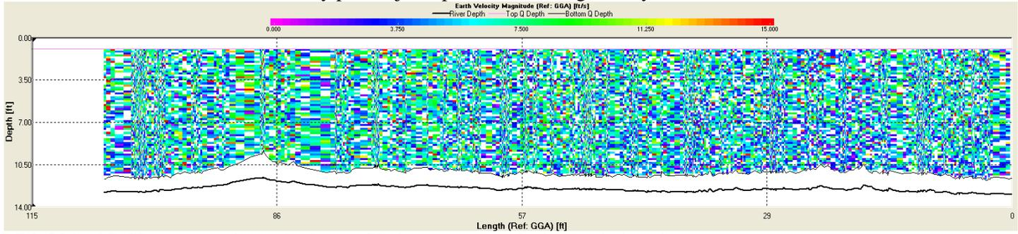
DB0-004. ADCP cross section velocity profile just upstream the bridge in bay 1
