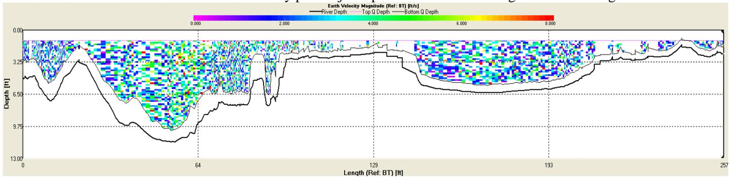
ESBS@MB 1-000. ADCP cross section velocity profile just upstream gates during flow monitoring
