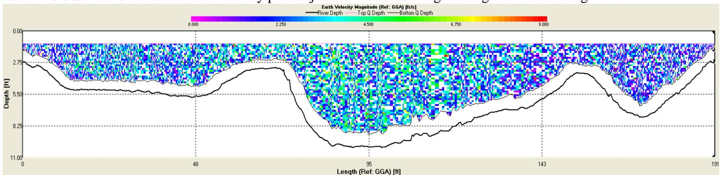
ESBRW1-002. ADCP cross section velocity profile just upstream weir during flow monitoring
