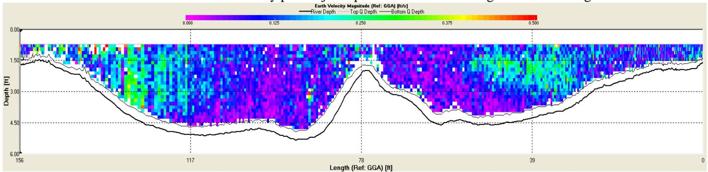
SLWRLFX1-000. ADCP cross section velocity profile just upstream the road during flow monitoring
