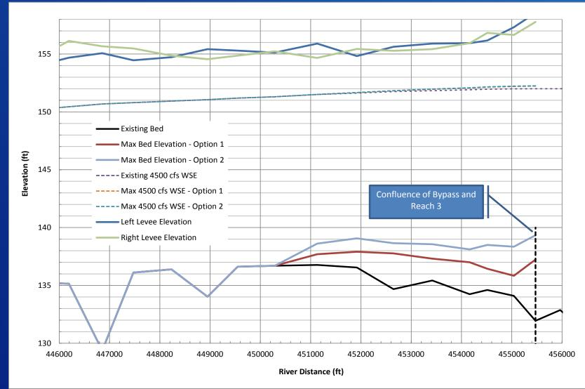
Simulations do not indicate that 4500 cfs will encroach into the 3 feet of freeboard
