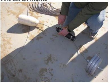
fish be reported to the contacts listed at the end of this advisory. Each sensor is weighted to keep it submerged and includes a buoy to keep it vertical in the river (see picture at right). The information collected through the study will support spring-run and fall-run Chinook salmon reintroduction decisions in the future.
