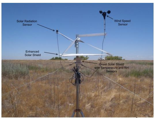
Figure 2. Weather Station with an enhanced solar shield constructed of a 2 ft<sup>2</sup> 1/8-inch plywood sheet painted white, an Onset solar shield with temperature and relative humidity sensors, a solar radiation sensor, and wind speed sensor in a non-forested site on the San Luis National Refuge.
